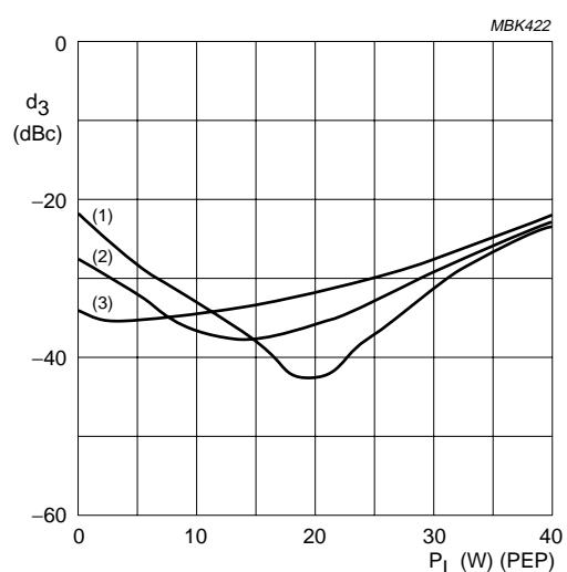
$V_{CE} = 26$  V;  $f_1 = 1950$  MHz;  $f_2 = 1950.1$  MHz.
