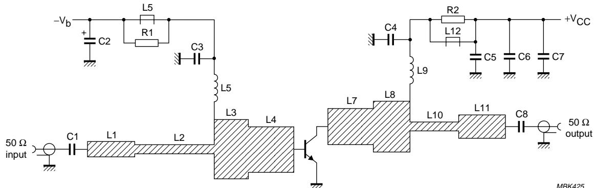
Fig.1 Class-AB testcircuit for 1.8 to 2 GHz.
