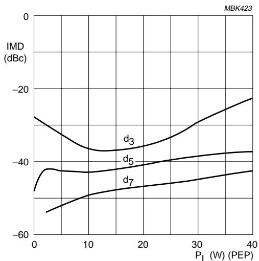
$V_{CE} = 26$  V;  $I_{cq} = 80$  mA;  $f_1 = 1950$  MHz;  $f_2 = 1950.1$  MHz.
