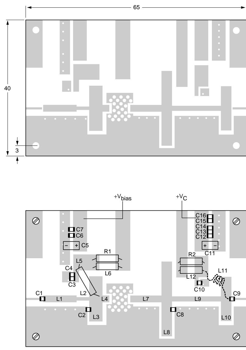
Fig.2 Printed-circuit board and lay-out amplifier.
