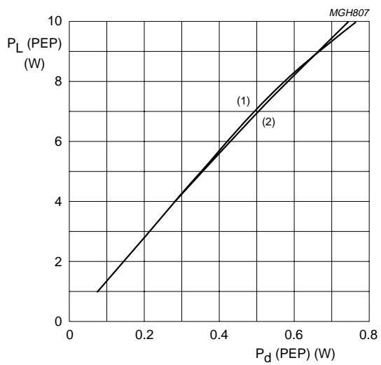
(1)  $f = 960$  MHz.(2)  $f = 935$  MHz.Class AB:  $V_{ce} = 26$  V,  $I_{cq} = 25$  mA, 9 W PEP loadline  $\Delta f = 0.1$  MHz,  $f_1 = 960.1$  MHz.Fig.5 BLV909 PL-PEP = f ( $P_d$ ).
