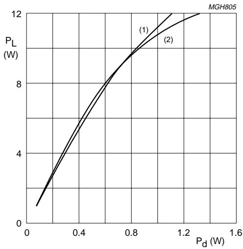
(1)  $f = 960 \text{ MHz}$ .(2)  $f = 935 \text{ MHz}$ .Class AB:  $V_{ce} = 26 \text{ V}$ ,  $I_{cq} = 25 \text{ mA}$ , 9 W loadline,  $f = 960 \text{ MHz}$ .Fig.3 BLV909  $P_L = f(P_d)$ .
