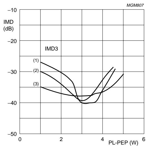
Class AB:  $V_{ce} = 26$  V;  $I_{cq} = 15$  mA; 4 W PEP loadline;  $\Delta f = 0.1$  MHz.
