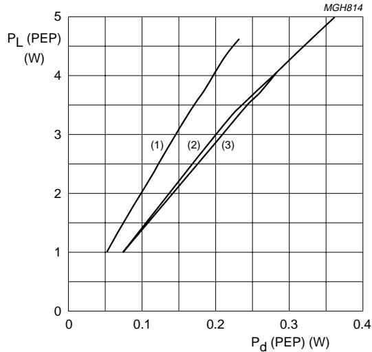
Class AB:  $V_{ce} = 26$  V;  $I_{cq} = 15$  mA; 4 W PEP loadline;  $\Delta f = 0.1$  MHz.
