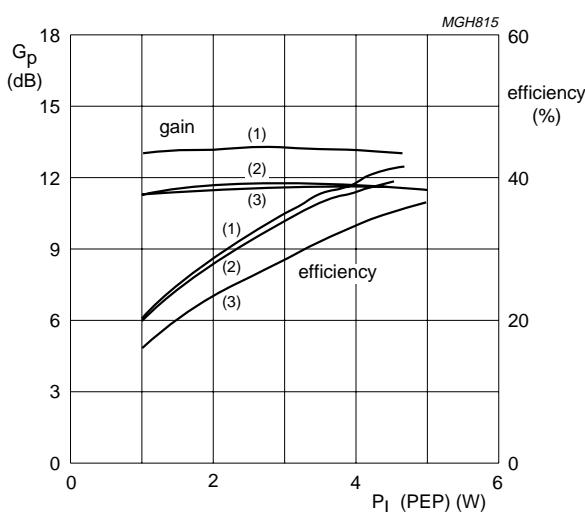
Class AB:  $V_{ce} = 26$  V;  $I_{cq} = 15$  mA; 4 W PEP loadline;  $\Delta f = 0.1$  MHz.
