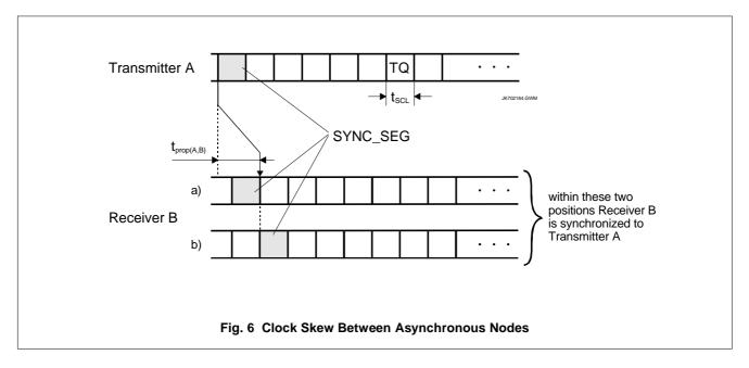
sents the worst case condition for accumulated phase error during normal communication. This phase error has to be compensated by the programmed Synchronization Jump Width (SJW) and defines the conditions for the minimum value of SJW.
