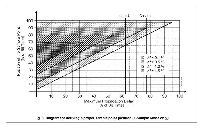
Fig. 8 may be used to derive the range for a proper sample point position for a certain requested maximum propagation delay also expressed in percent of the bit time period. For example, assuming an oscillator tolerance of 0.5% and a maximum propagation delay of 62,5% of the bit period as indicated for case b, the sample point position has to be in the range between 75% and 90% of the bit time. With the help of Equation (30), the corresponding range for TSEG2 can be calculated.
