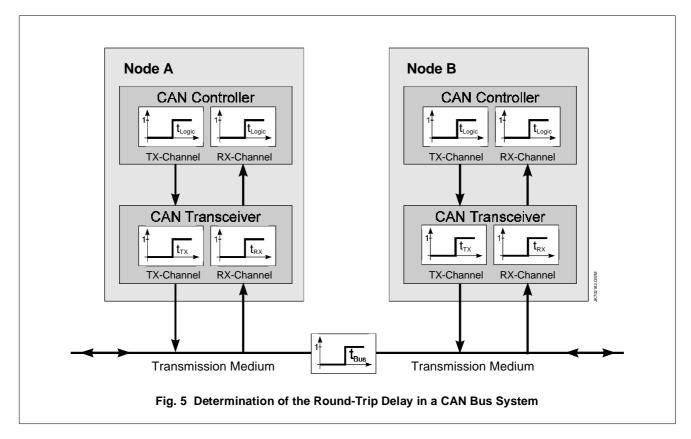
Normally, an effective maximum loop delay,  $t_{loop.eff}$ , is specified in the data sheets of controllers and transceivers. As an example, according to Fig. 5, the effective loop delay of a transceiver calculates as follows:
