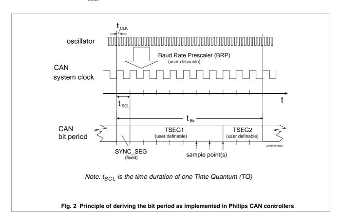
Another time segment of importance to CAN bit timing calculations is the Synchronization Jump Width (SJW), with time duration t<sub>SJW</sub>. The SJW segment is not a segment of the bit period but rather defines the maximum number of TQ by which a bit period can be lengthened or shortened in the event of resynchronization.
