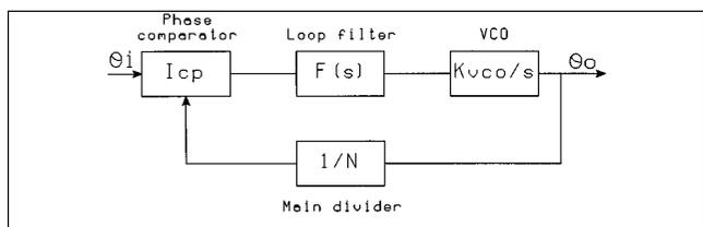
**Figure 5-2. Block Diagram of a Phase Locked Loop**
