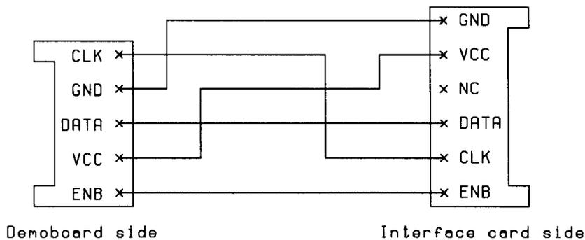
Figure 5-8. Interface Card PCB Layout and Cable Connection
