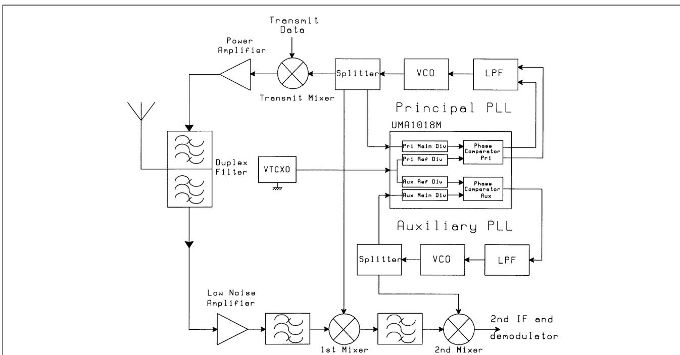
Figure 1-2. UMA1018M: Typical Application Block Diagram
