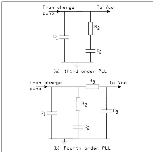
**Figure 3-2. Different Types of Passive Loop Filter**
