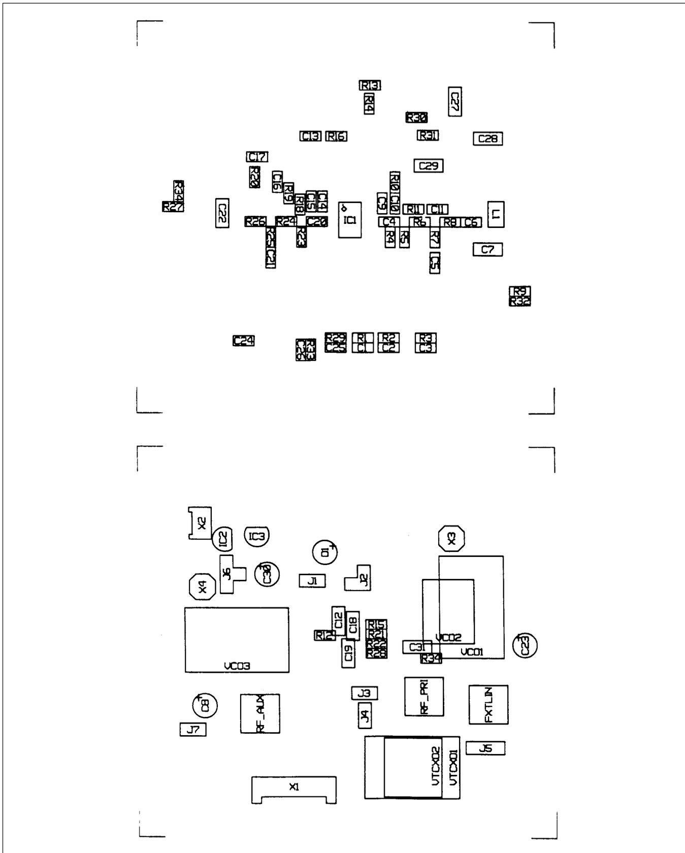
Figure 5-5. Demonstration Board Placement of Components
