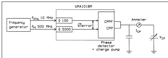
Figure 2-6. UMA1018M Principal Synthesizer Phase Detector Linearity Measurement
