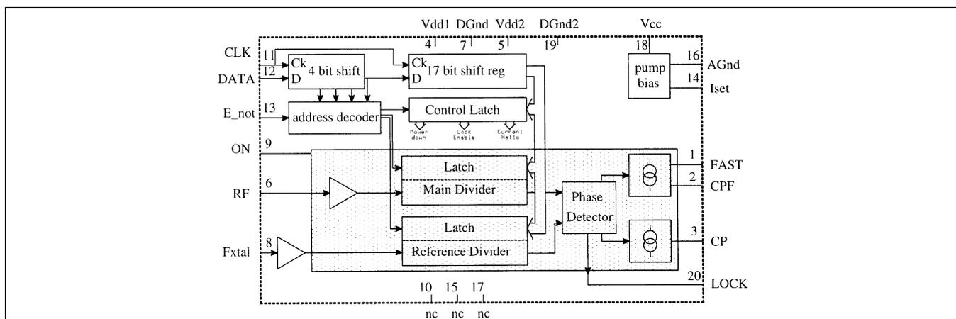
Figure 1–3. UMA1017M and UMA1019M/UMA1019AM Block Diagram
