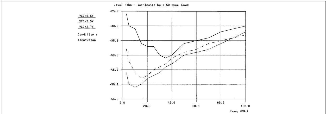
Figure 2-12. Reference Divider Input Sensitivity vs Frequency
