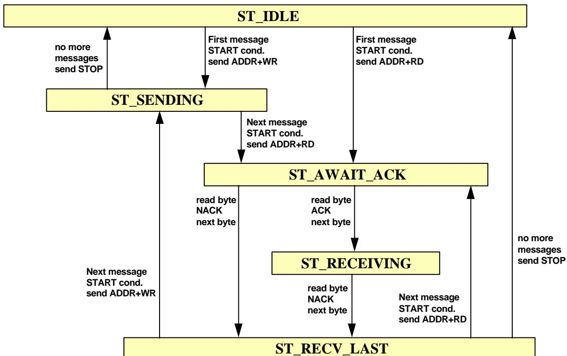
Figure 1. State transition diagram of the master state handler.
