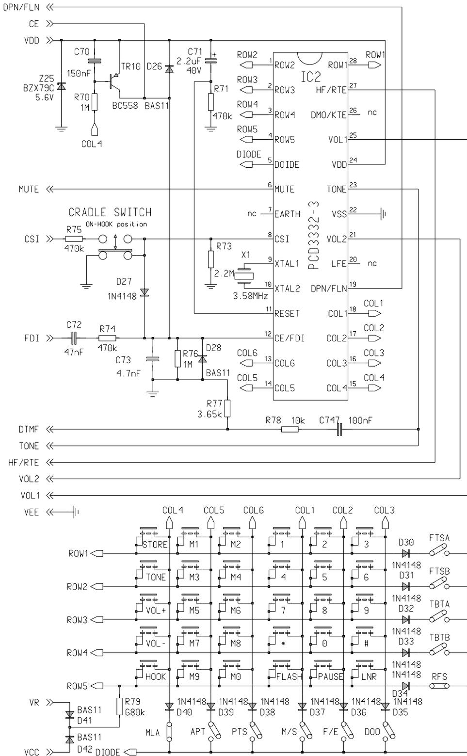
Fig.53 Application example 2; dialler/ringer PCD3332-3
