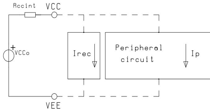
Fig.12 VCC supply point: equivalent schematic
