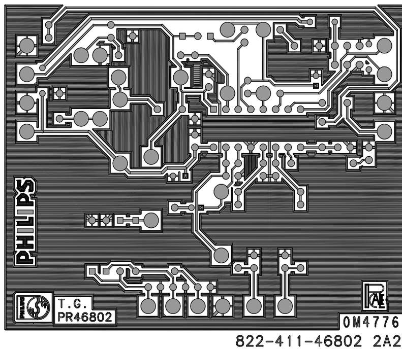
Fig.59 Layout of the wiring of the OM4776
