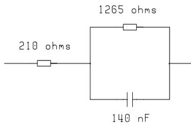
Fig.44 Equivalent average line impedance
