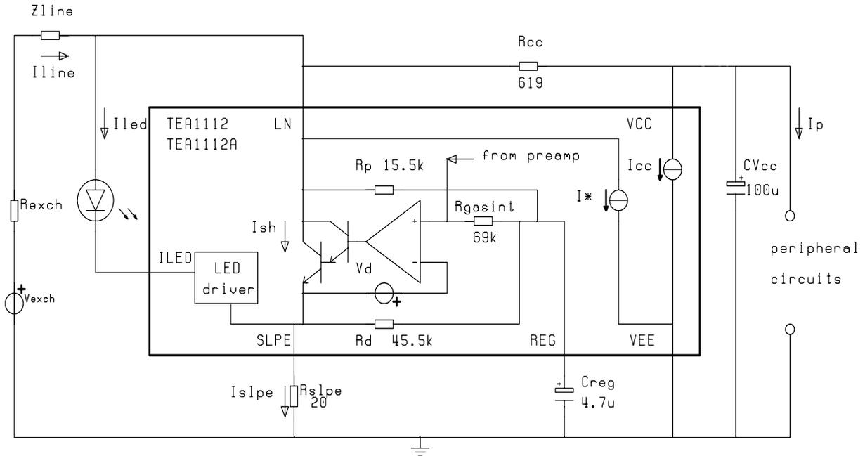
Fig.5 Supply configuration
