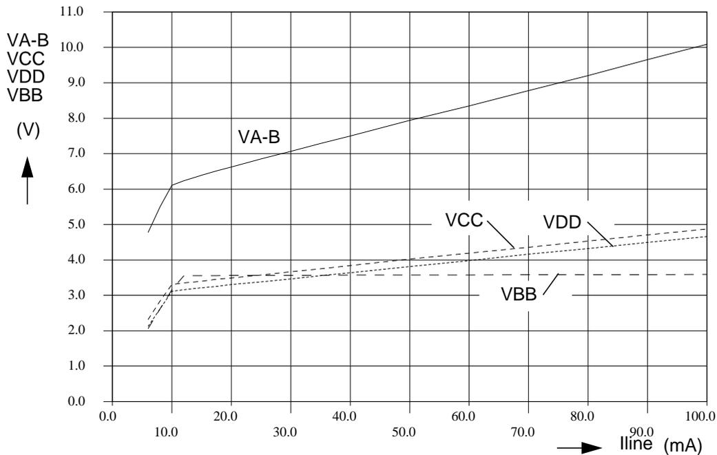
Fig.55 Voltages VA-B, VCC, VDD and VBB (with respect to SLPE) versus I<sub>line</sub>
