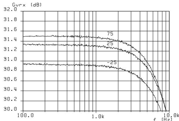
Fig.31 Receiving gain versus frequency: influence of temperature
