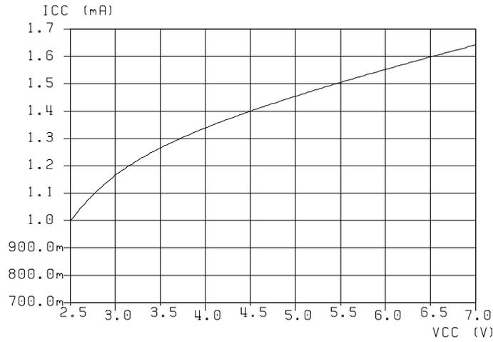
Fig.6 ICC versus VCC
