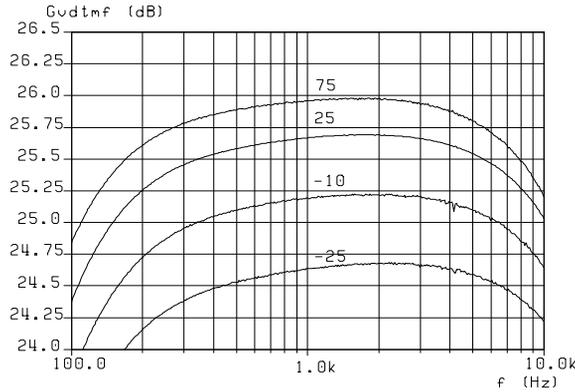
Fig.37 DTMF gain versus frequency: influence of temperature
