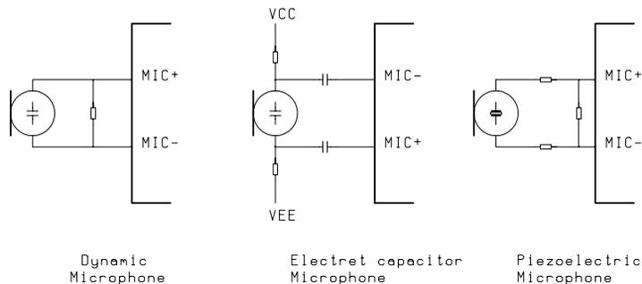
Fig.17 Microphone arrangements examples
