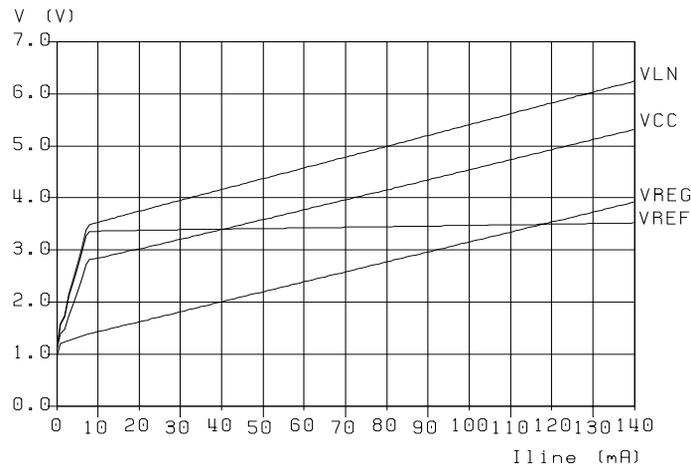
Fig.7 Main voltages versus line current
