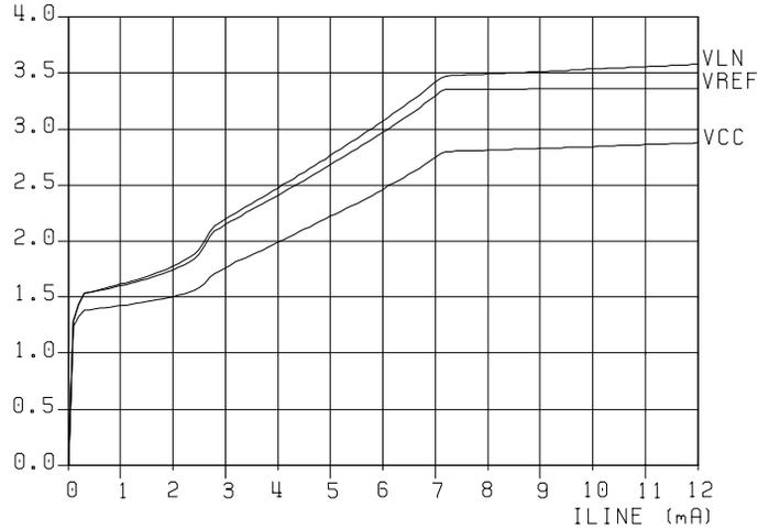
Fig.8 Low voltage behaviour
