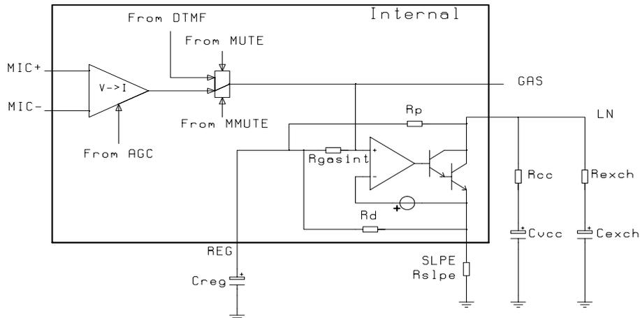
Fig.16 Microphone channel
