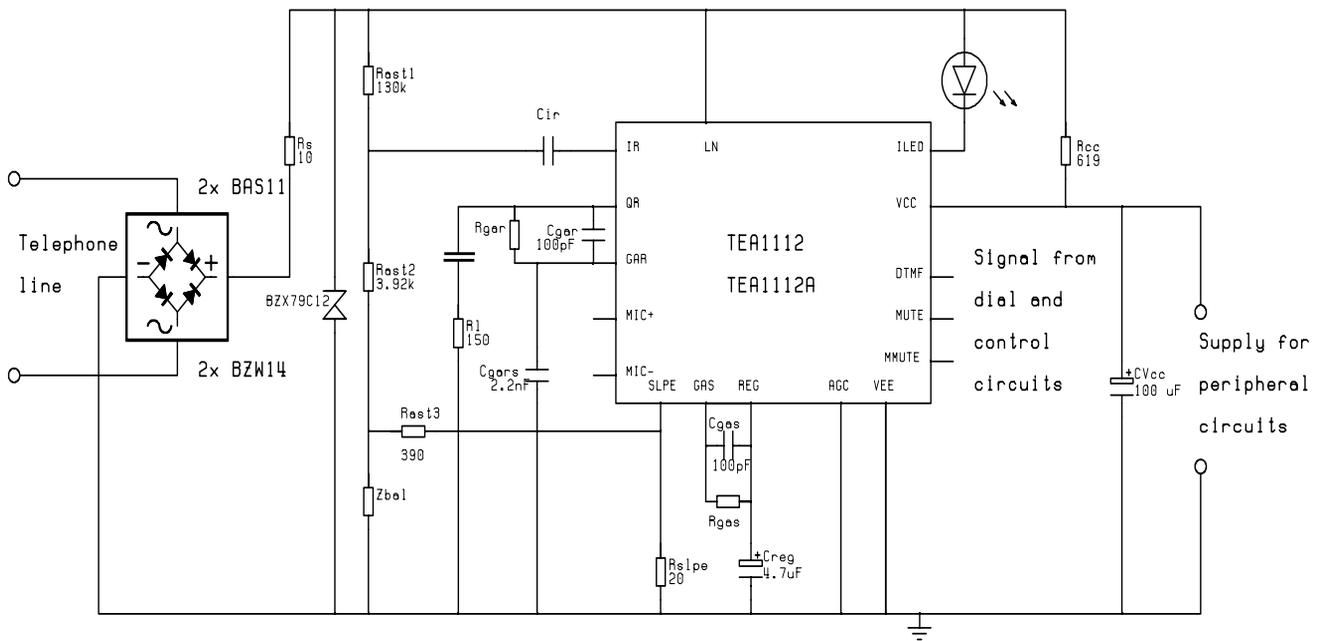
Fig.4 Basic application used for measurement
