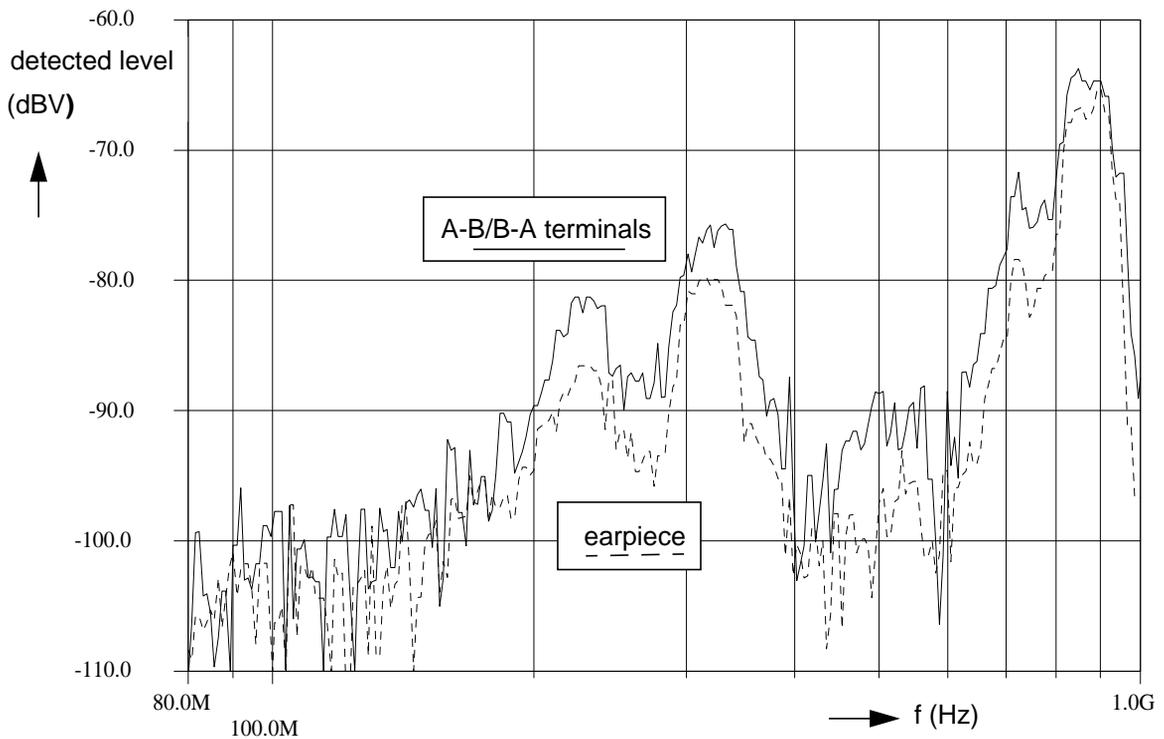
Fig.61 EMC behaviour of the OM4776; radiation test
