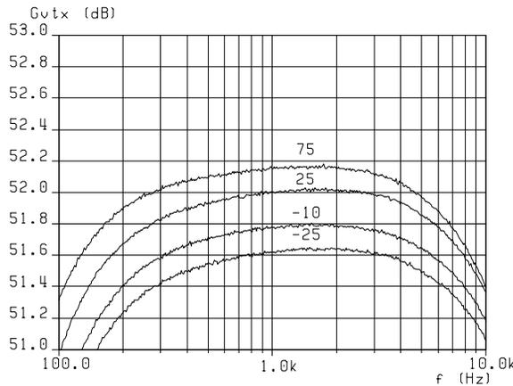
Fig.19 Microphone gain versus frequency: influence of temperature
