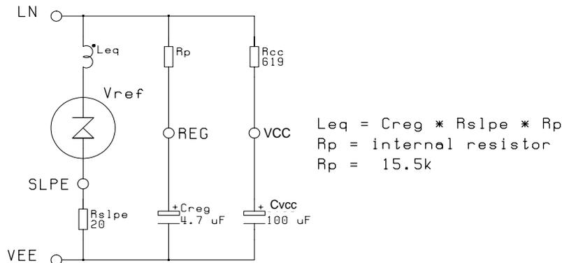
Fig.13 Equivalent set impedance
