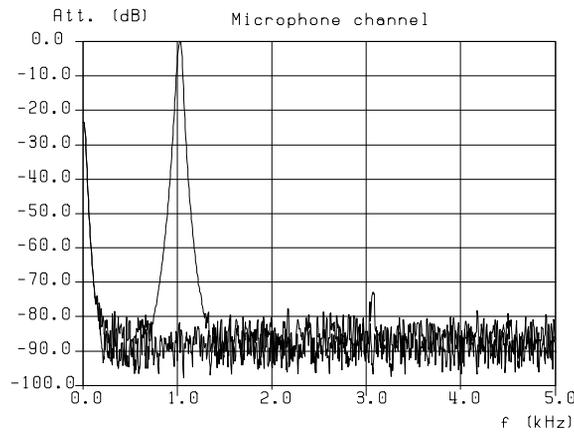
Fig.27 Microphone gain reduction in  $\overline{\text{MMUTE}}$  condition
