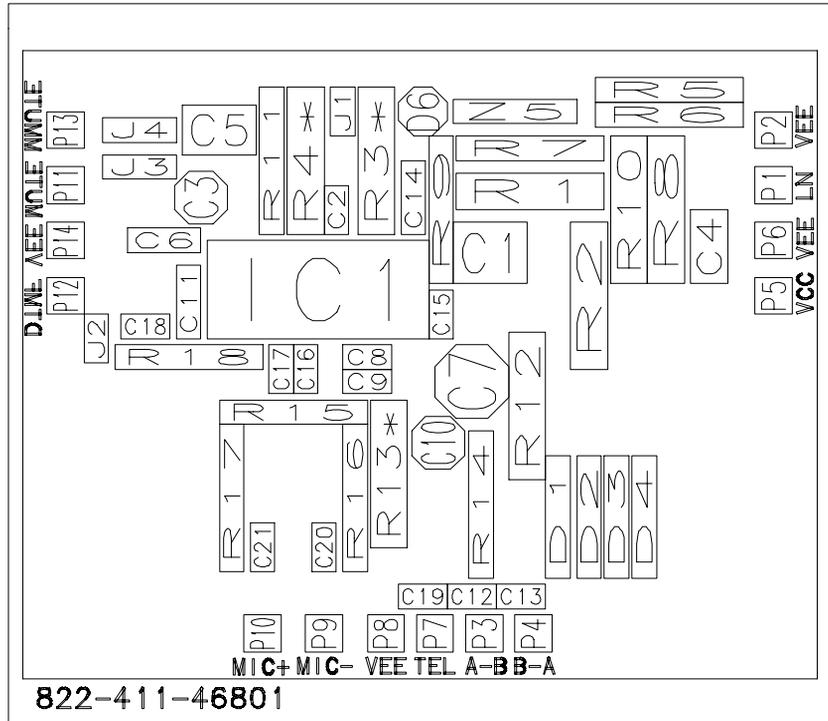
Fig.58 Components side of the OM4776 evaluation board
