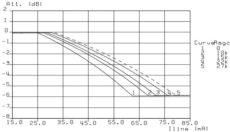
Fig.35 Automatic gain control on the microphone amplifier
