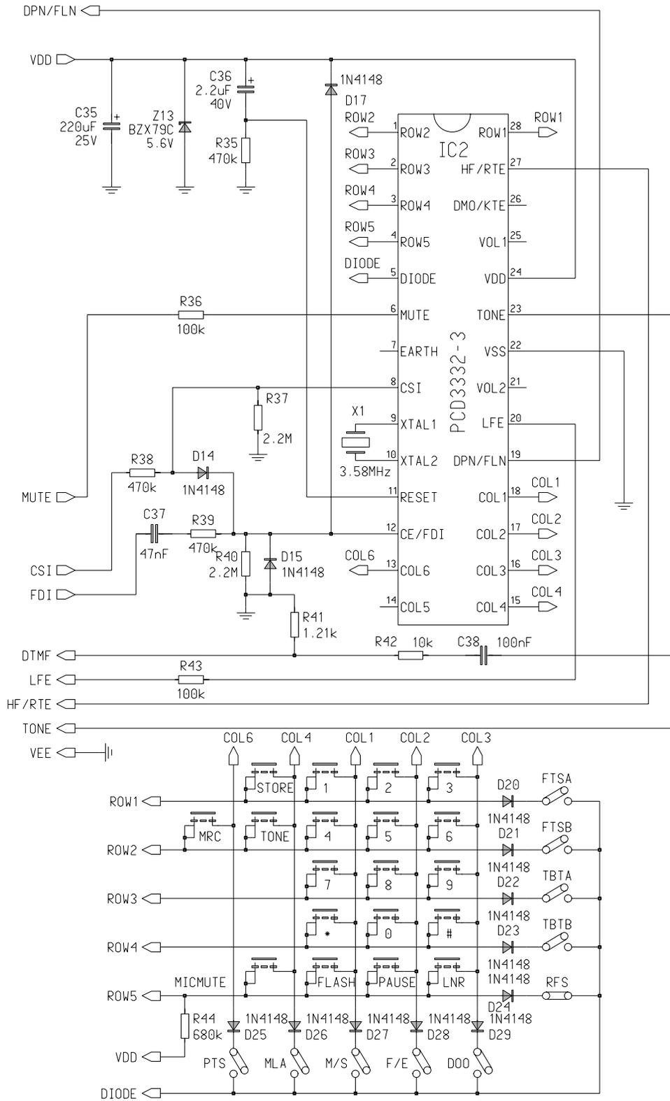
Fig.46 Application example 1; dialler/ringer PCD3332-3
