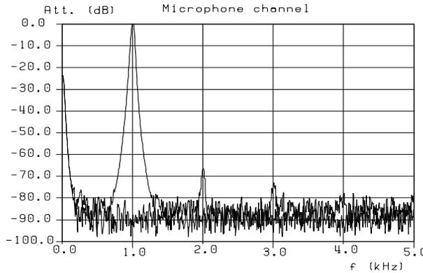
Fig.25 Microphone gain reduction in MMUTE condition
