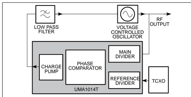
Figure 1. PLL Circuit Block Diagram
