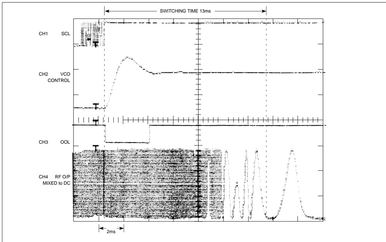
Figure 10. Typical Switching Waveforms
