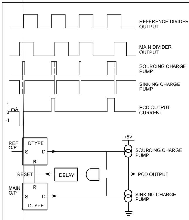
Figure 2. Digital Phase Comparator Operation
