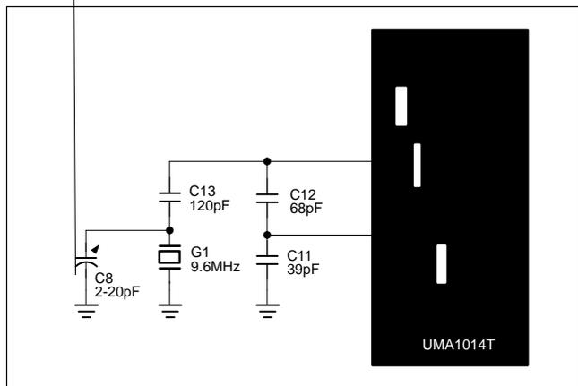
Figure 3. Crystal Oscillator Circuit Diagram
