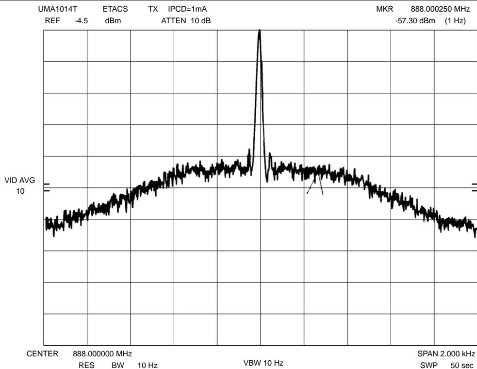
Figure 8. Typical Carrier Spectrum – 2kHz Span
