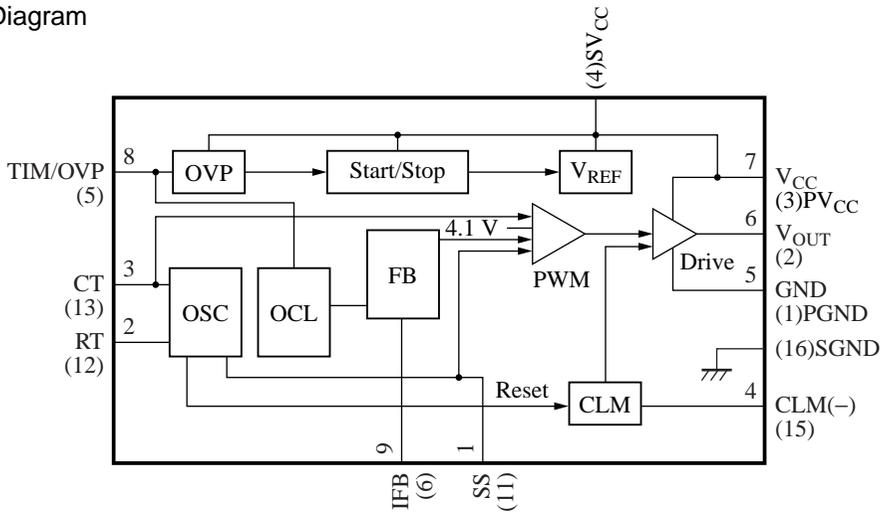
Note) The number in ( ) shows the pin number for the AN8022SB.
