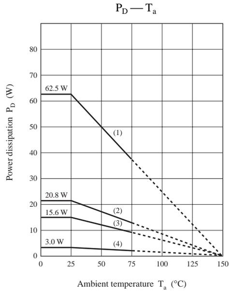
1.  $T_C = T_a, 62.5 \text{ W} (\theta_{j-c} = 2 \text{ } ^\circ\text{C/W})$
