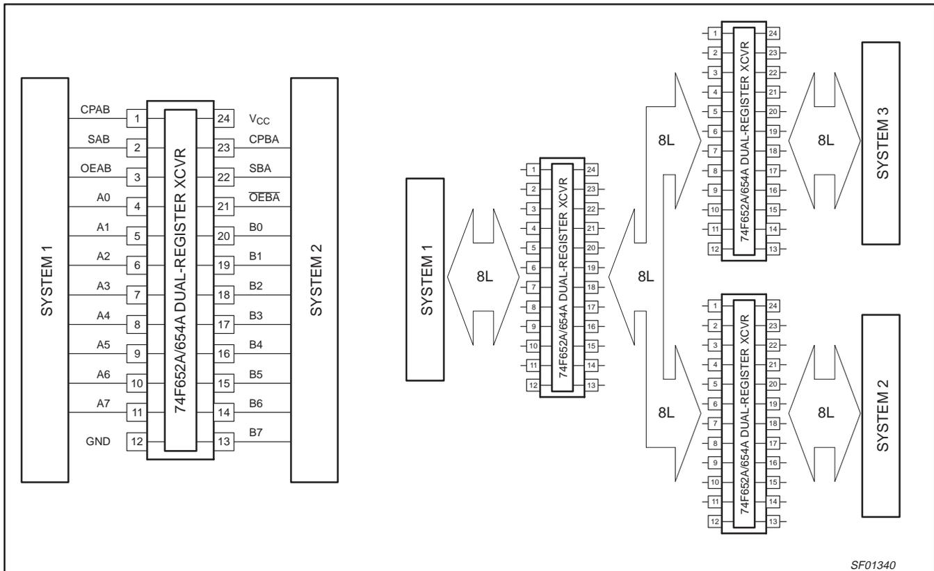
Figure 13. 74F Extended Octal-Plus Dual-Registered Transceiver Applications
