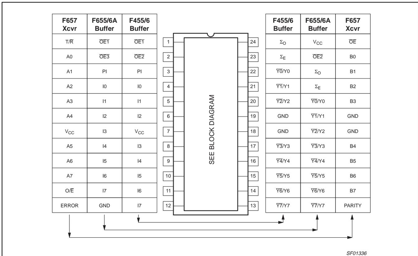
Figure 9. 74F Octal Parity Drivers/Transceiver Pin Configurations
