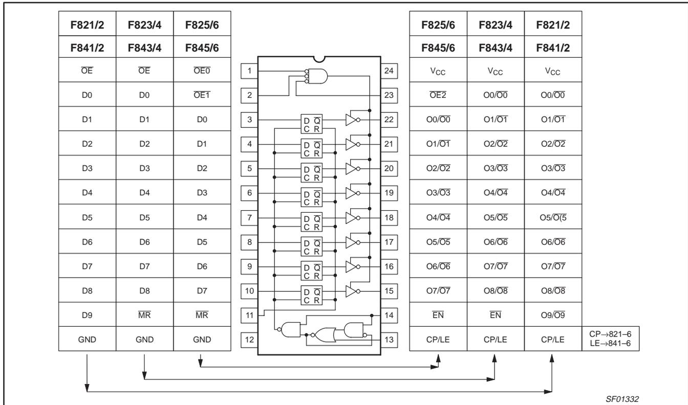
Figure 4. 74F82X and 74F84X Registered/Latched Buffer Pin Configurations
