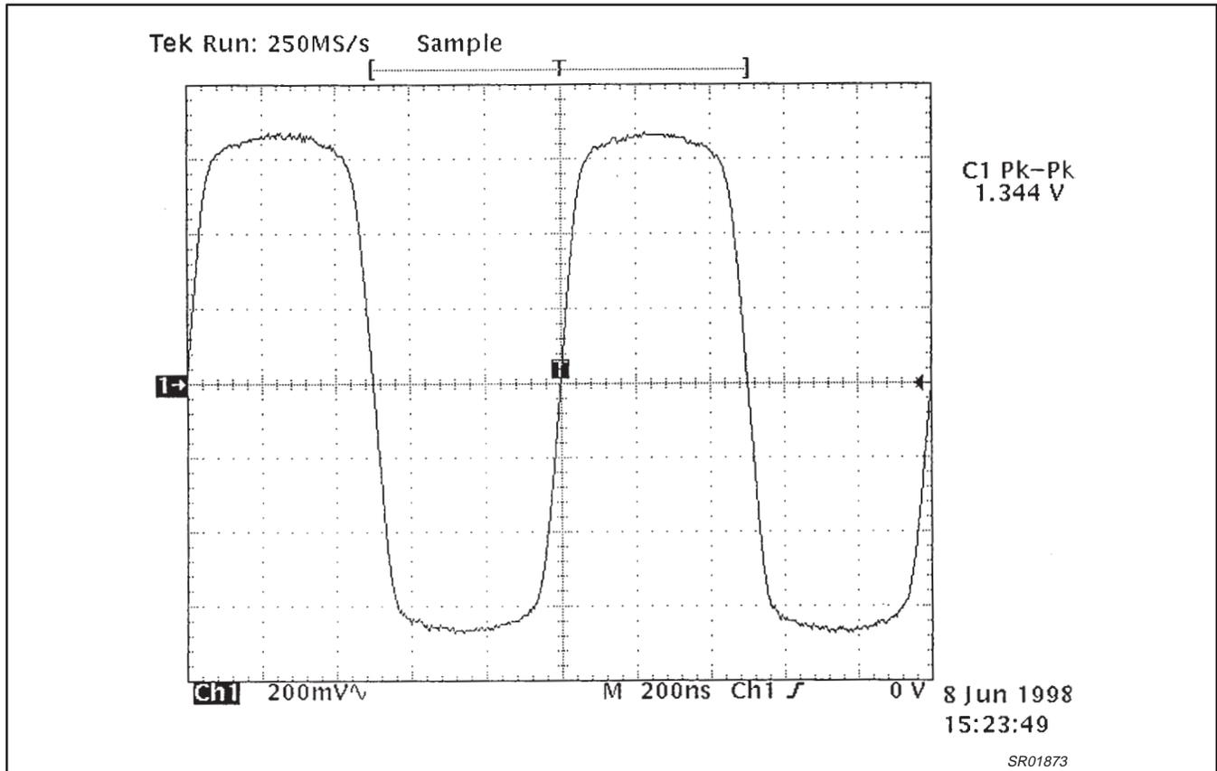
Figure 4. Symmetrical clamping at the Rx output when the Rx input is over-driven
