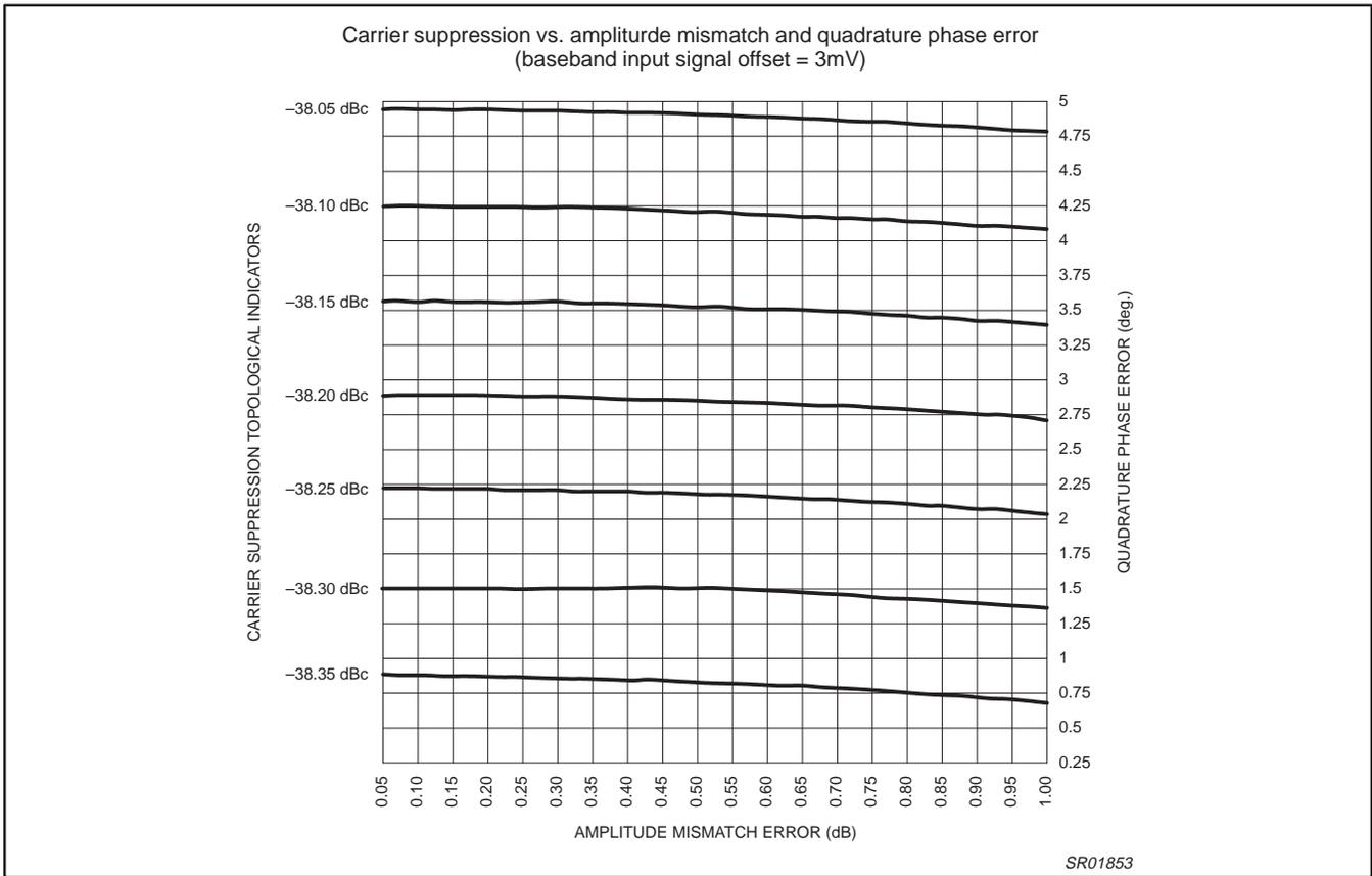
Figure 25. Carrier suppression vs. amplitude mismatch and quadrature phase error
