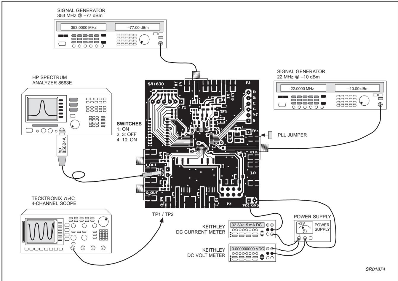
Figure 5. The set-up for measuring Rx harmonic distortion
