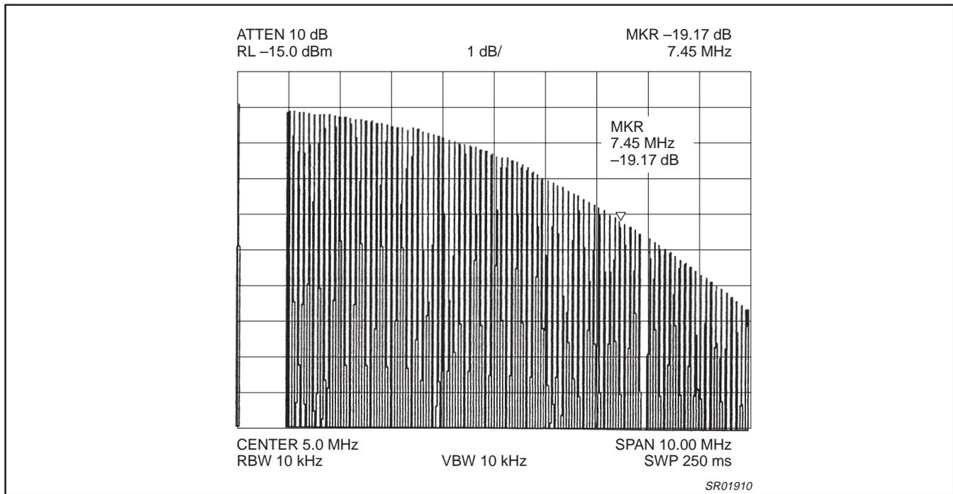
Figure 10. Rx 3 dB bandwidth measurement
