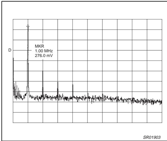
Figure 6. Voltage level of the Rx output fundamental
