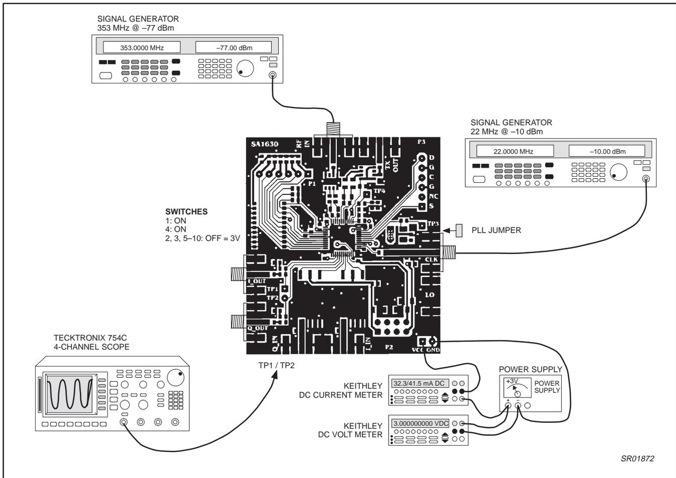
Figure 3. Set-up for Rx path voltage gain and symmetrical compression measurements
