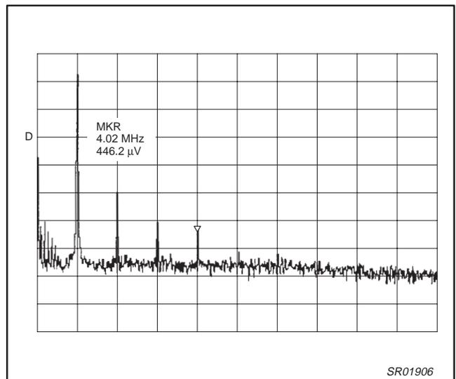
Figure 9. Voltage level of the Rx output 4th harmonic
