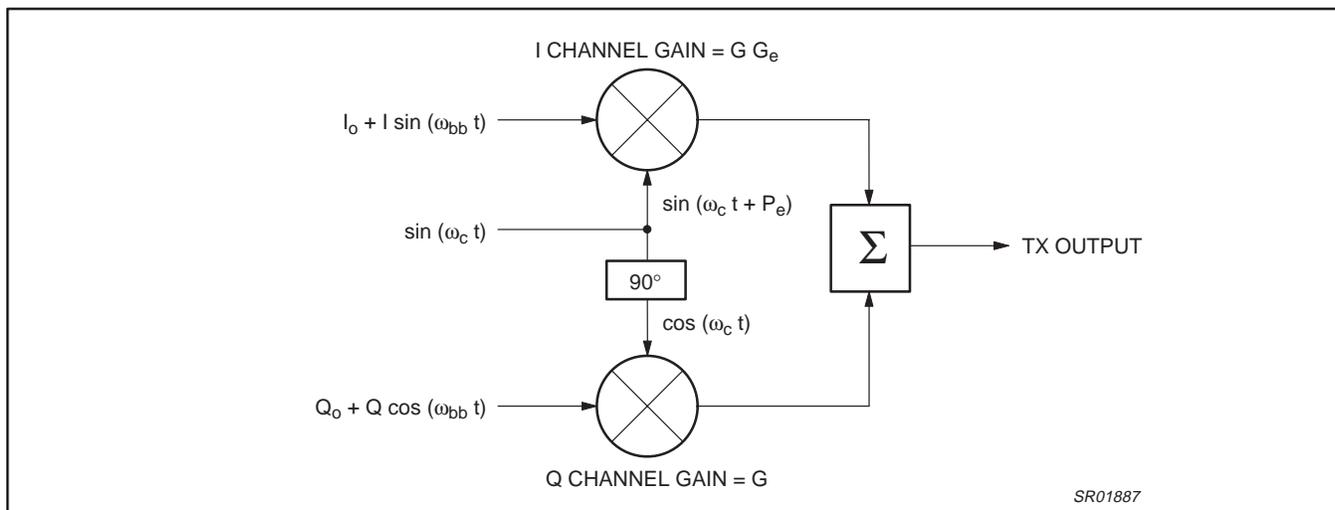
Figure 23. showing a conceptual schematic of I/Q modulation circuitry
