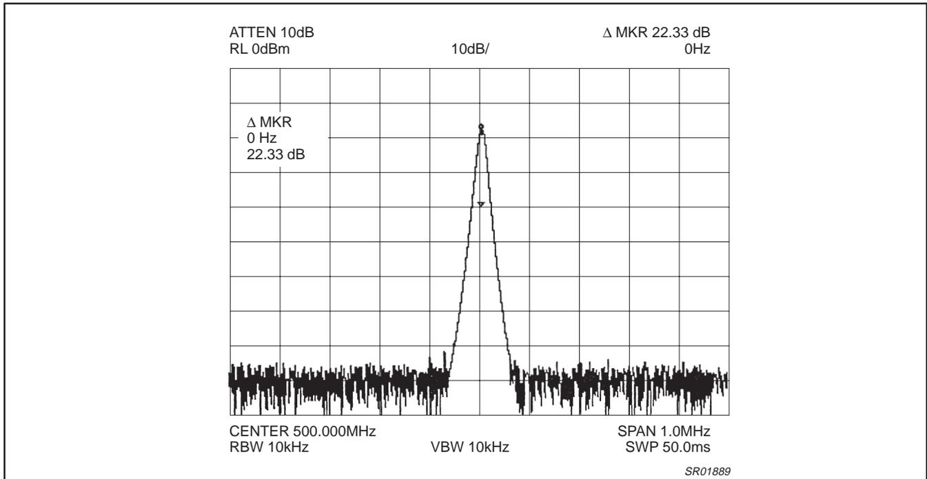
Figure 18. LNA gain of amplifier in Tx noise floor measurement set-up
