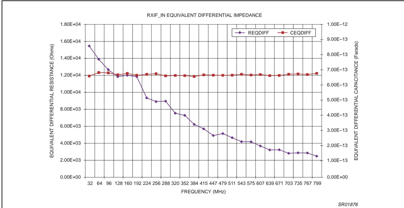
Figure 20. Rx input equivalent differential impedance variation over frequency
