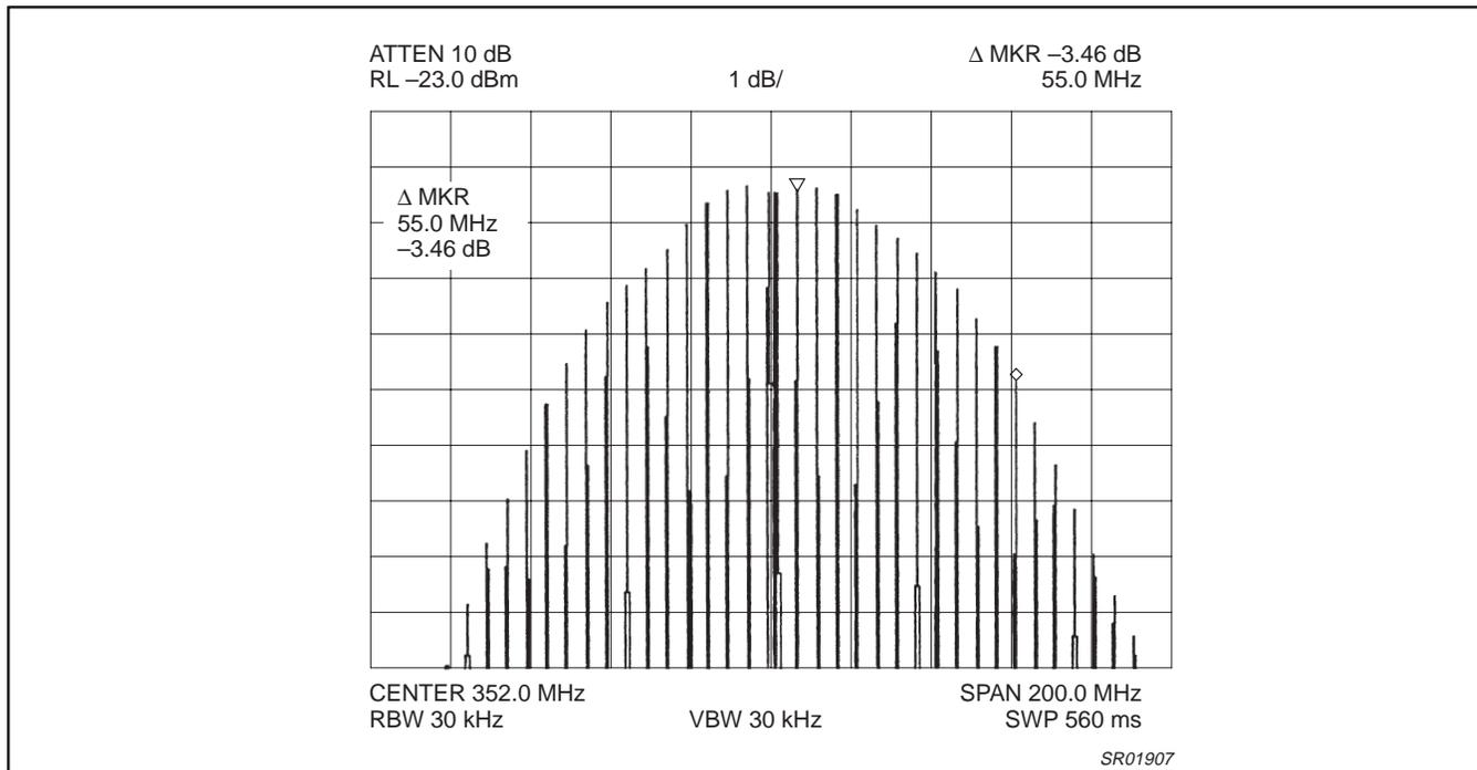
Figure 16. Tx input modulation bandwidth
