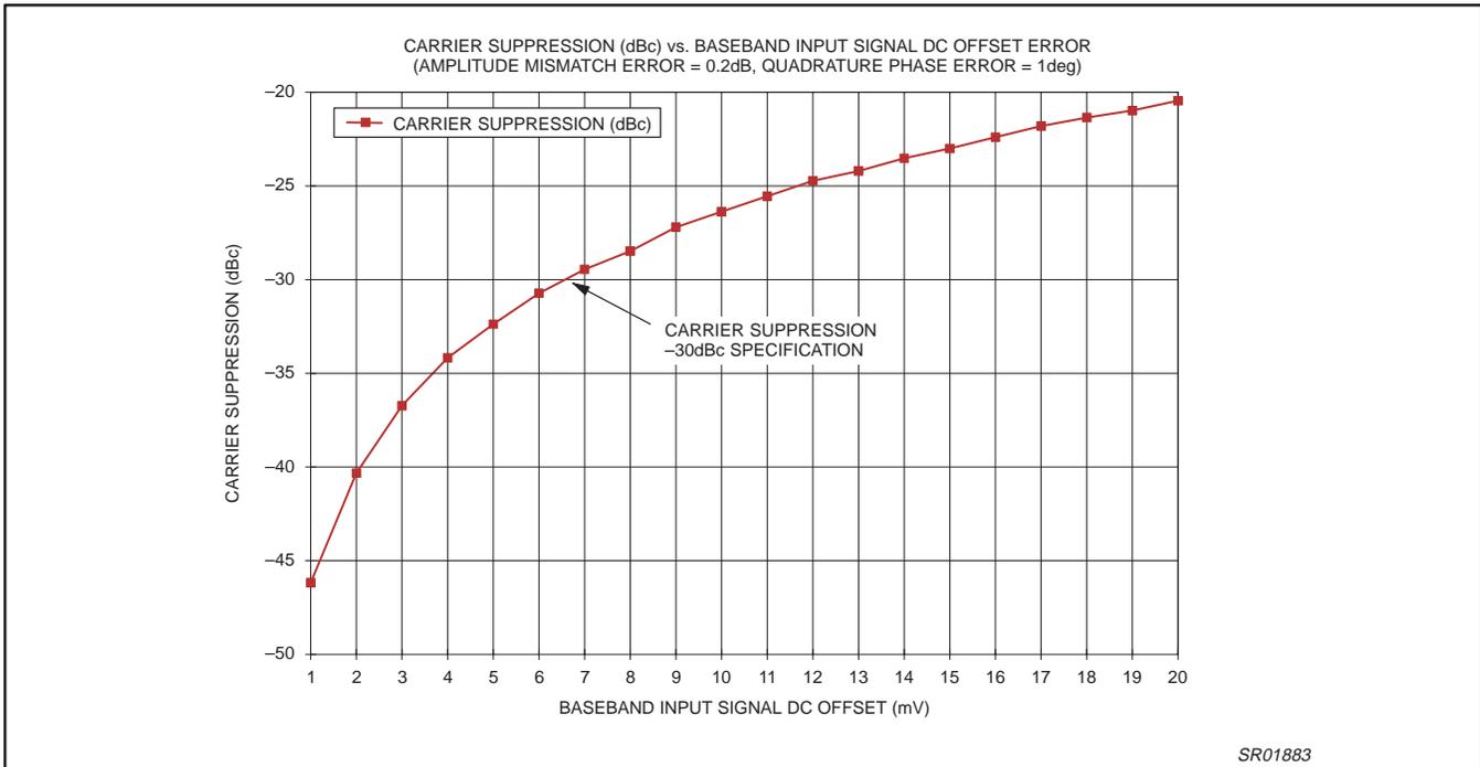
Figure 24. Carrier suppression as a function of baseband input signal DC offset
