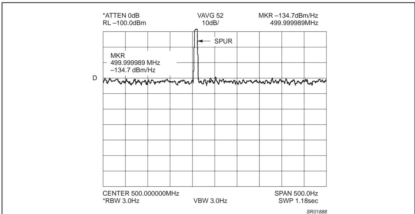
Figure 19. SA1630 Tx noise floor with 22.3 dB LNA in measurement system
