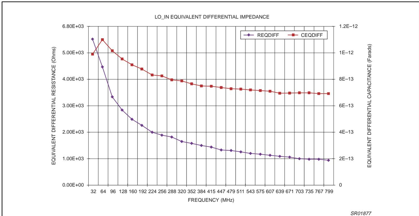
Figure 21. Tx output equivalent differential impedance variation over frequency
