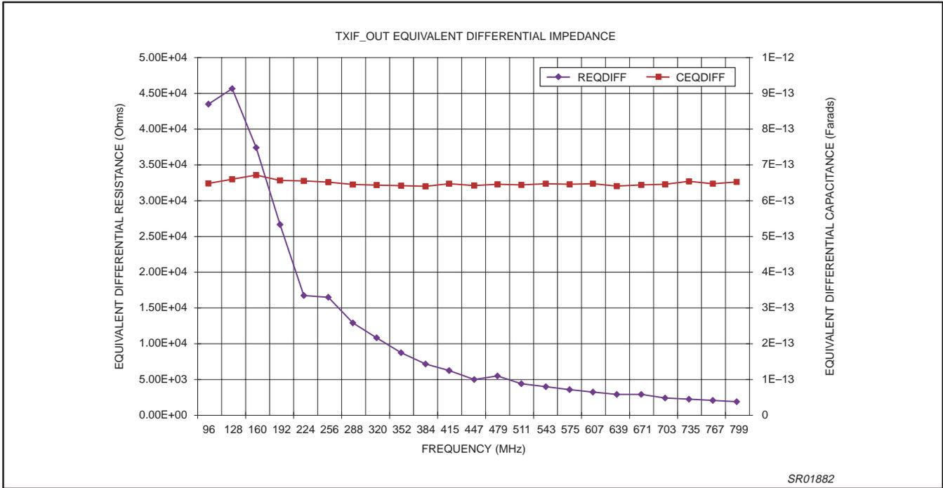
Figure 22. LO input equivalent differential impedance variation over frequency
