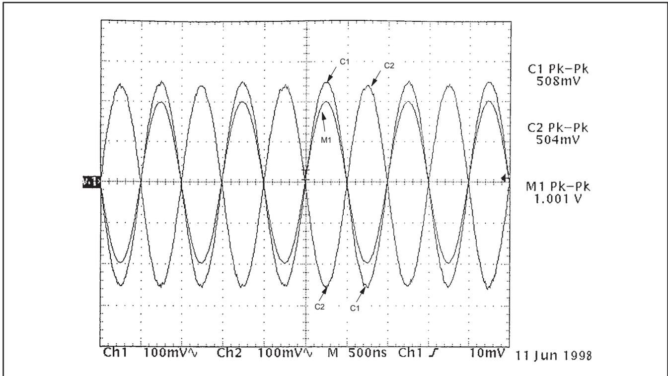
Figure 12. Calibrated 1V<sub>p-p</sub> signal at the Tx input pins
