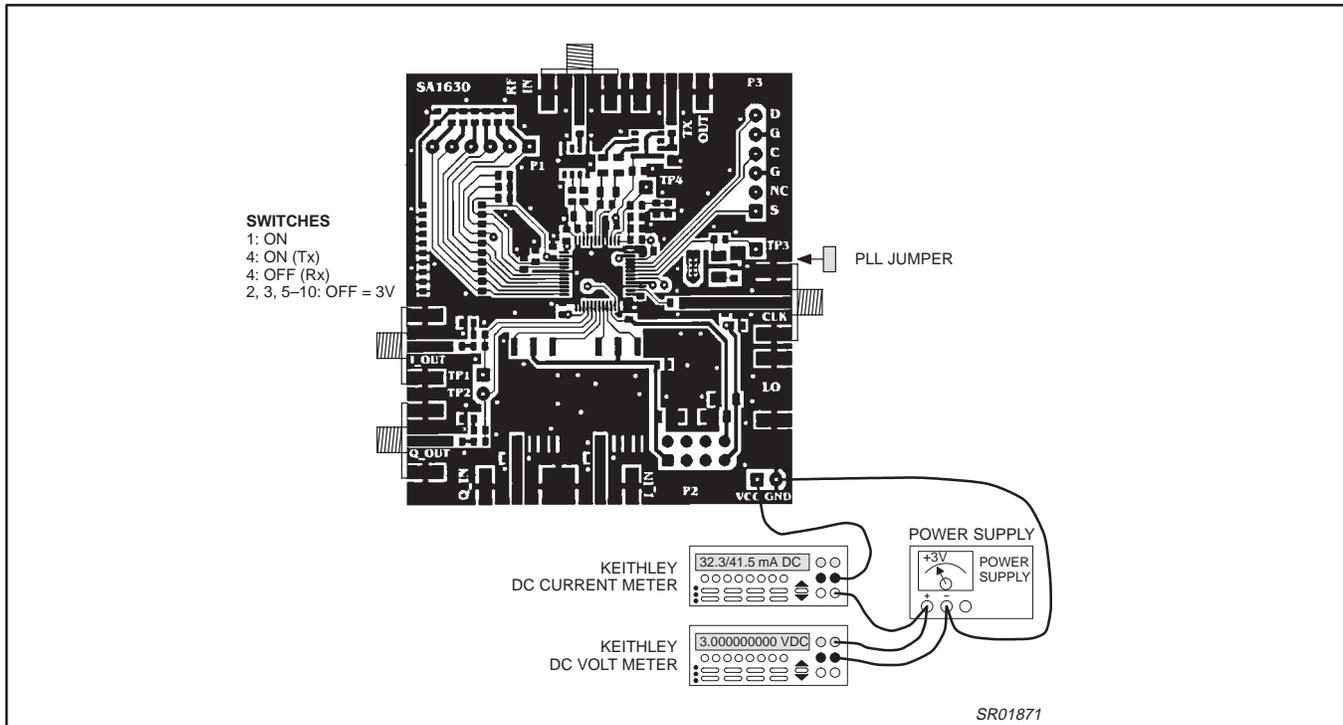
Figure 2. DC supply setup and mode select switch settings
