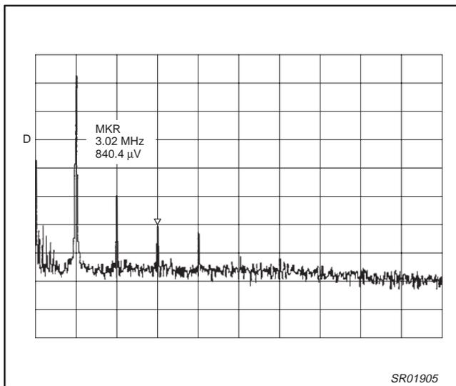
Figure 8. Voltage level of the Rx output 3rd harmonic
