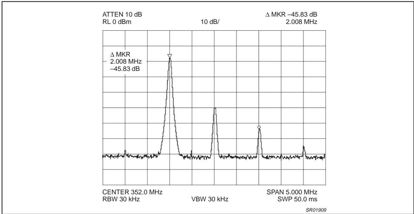
Figure 14. Tx output sideband suppression
