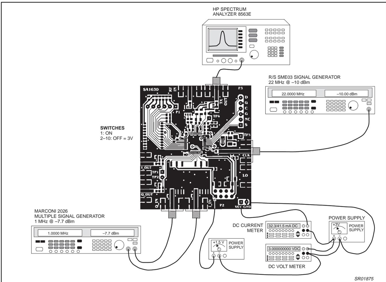
Figure 11. Tx measurement set-up
