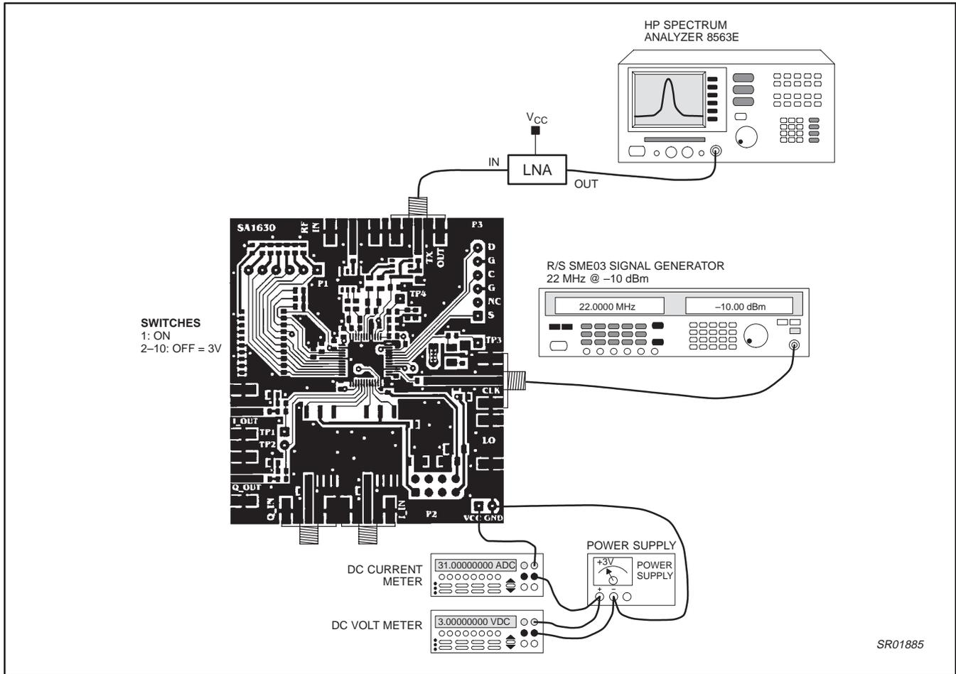
Figure 17. Tx noise floor measurement set-up
