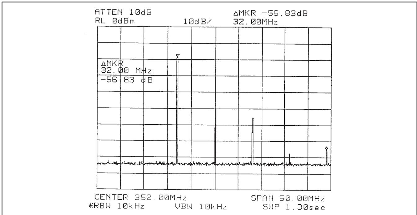
Figure 15. Tx output 3rd harmonic distortion
