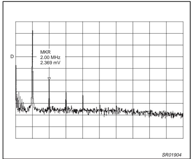
Figure 7. Voltage level of the Rx output 2nd harmonic
