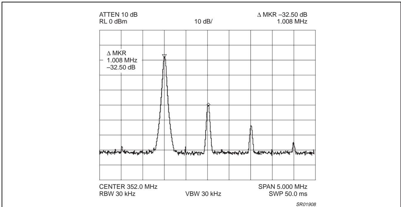
Figure 13. Tx output carrier suppression
