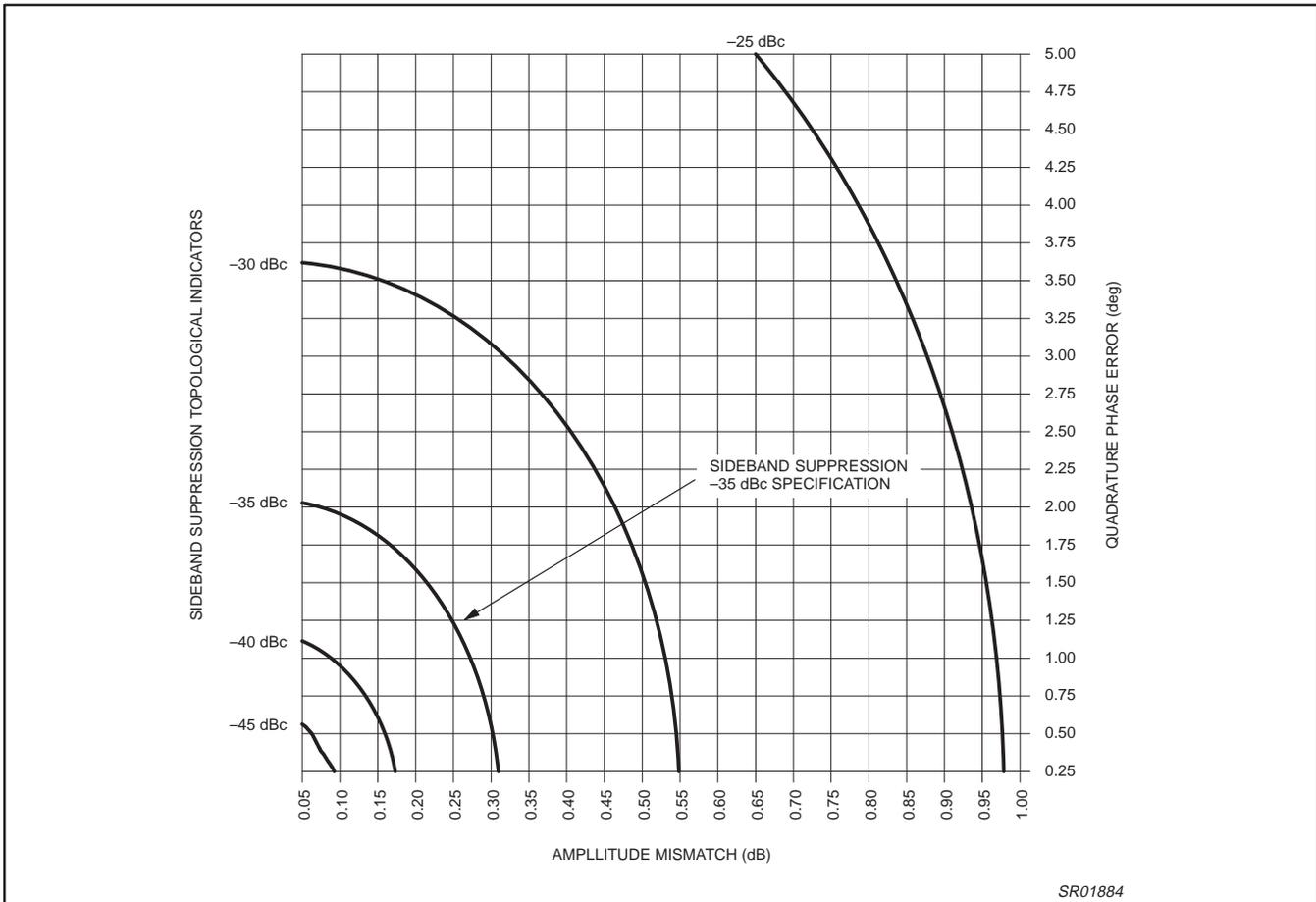
Figure 26. Sideband suppression vs. amplitude mismatch and quadrature phase error
