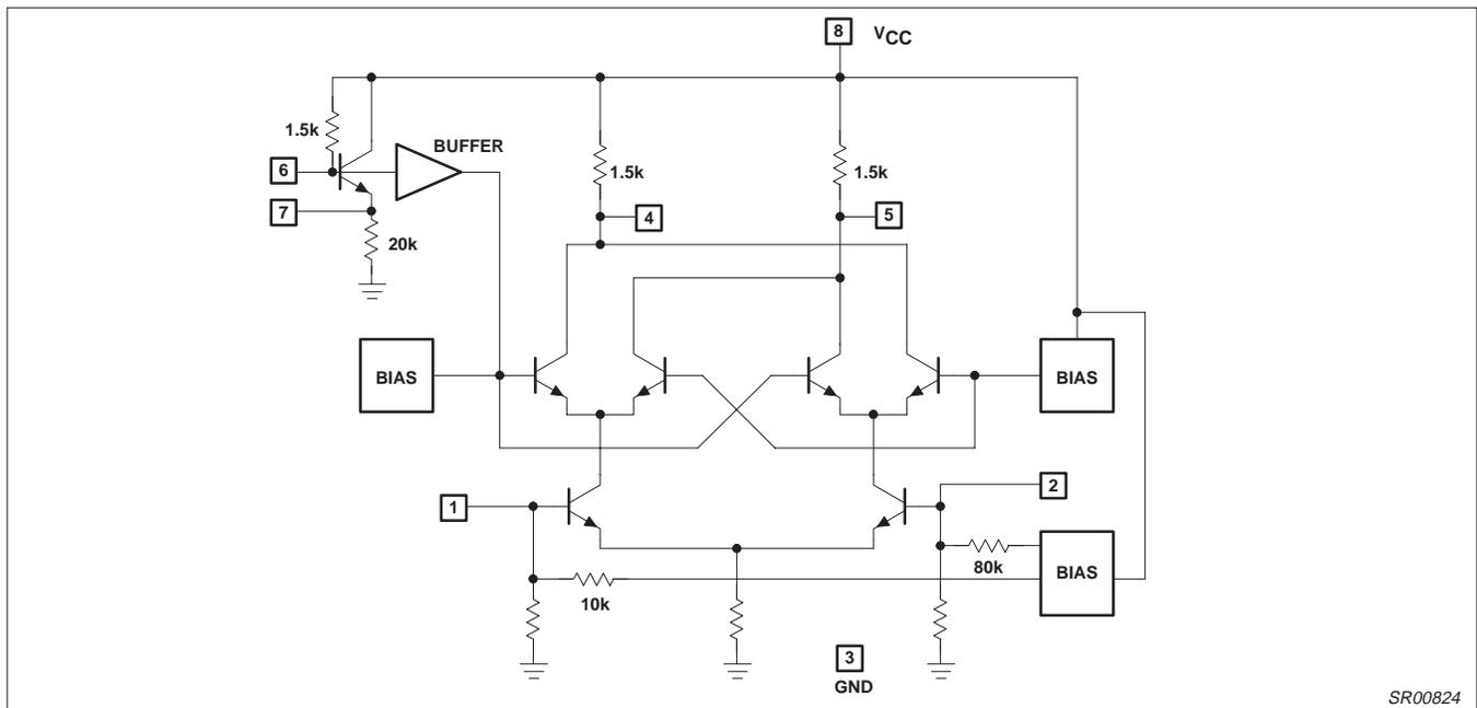
Figure 5. SA602 Equivalent Circuit
