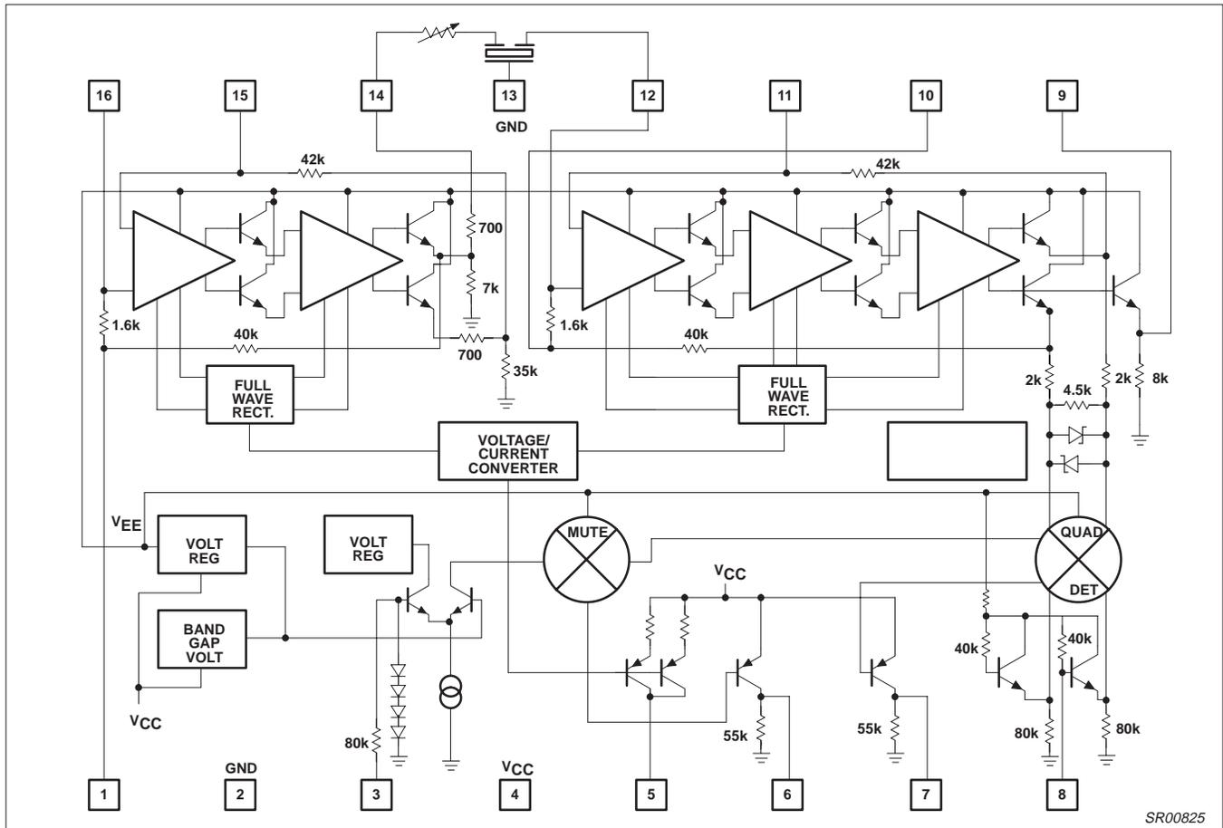
Figure 6. SA604A Equivalent Circuit
