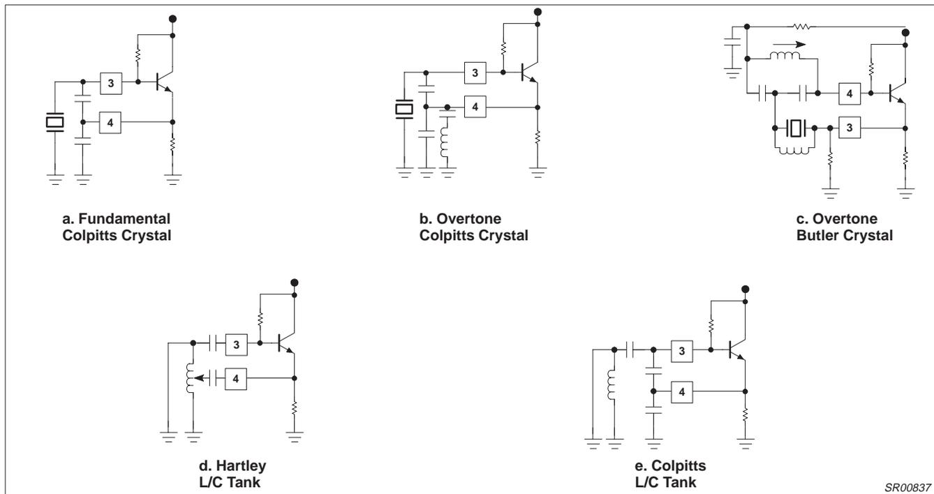
Figure 18. Oscillator Configurations
