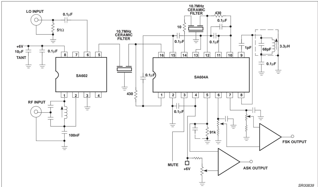
Figure 20. Basic SA602/604A Data Receiver
