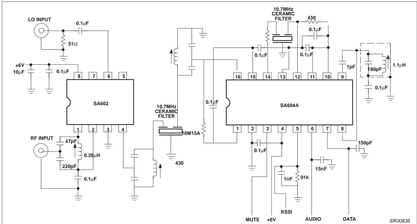
Figure 16. SA602/604A Demonstration Circuit with RF Input of 152.2MHz and IF of 10.7MHz ±7.5kHz
