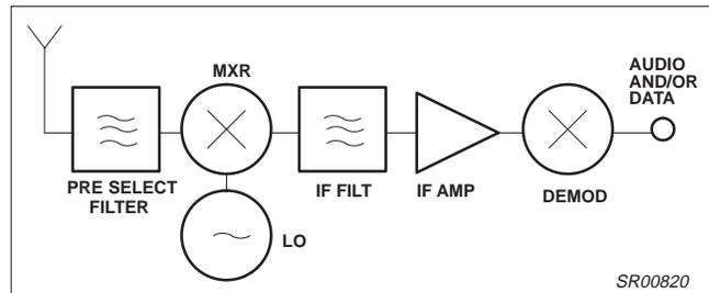
Figure 1. Basic Hetrodyne Receiver
