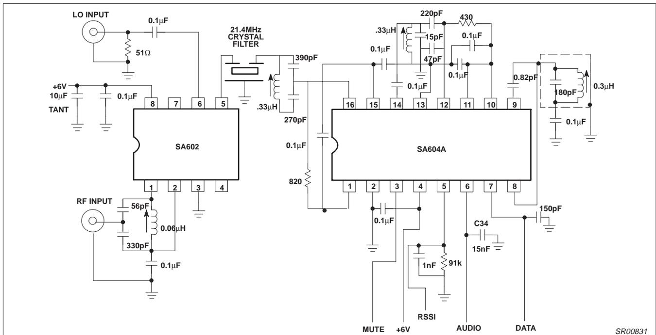
Figure 12. SA602/604A Demonstration Circuit with RF Input of 90MHz and IF of 21.4MHz ±7.5kHz
