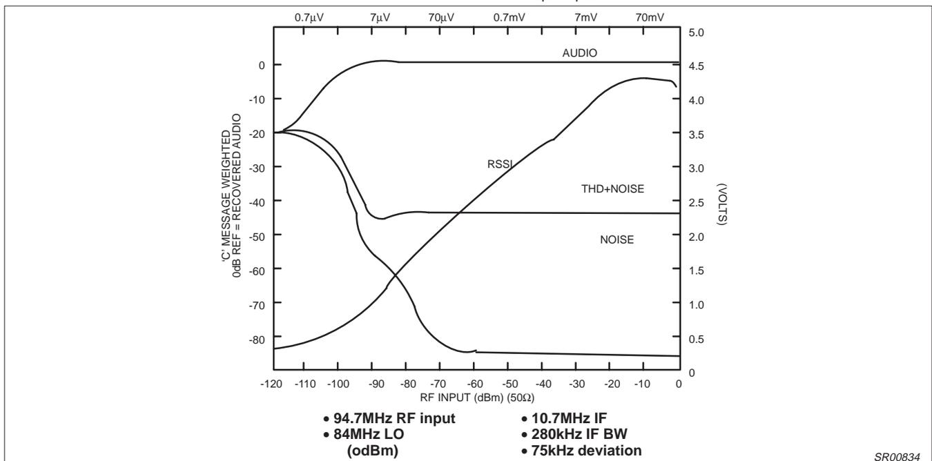
Figure 15. FM Broadcast Receiver (Wide Band)
