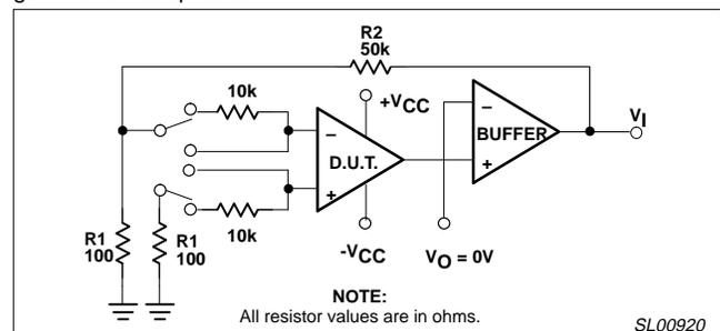
Figure 7. Circuit Diagram Used for CMRR Measurement
