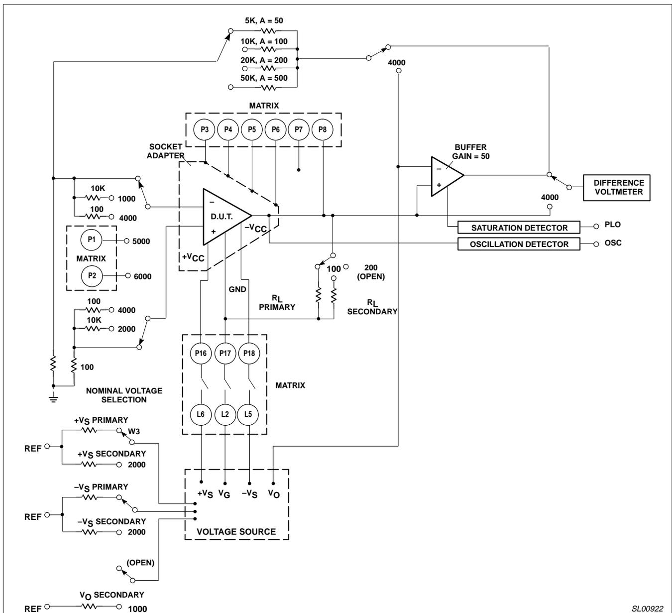
**Figure 9. A Typical Op Amp Test Circuit (Simplified)**
