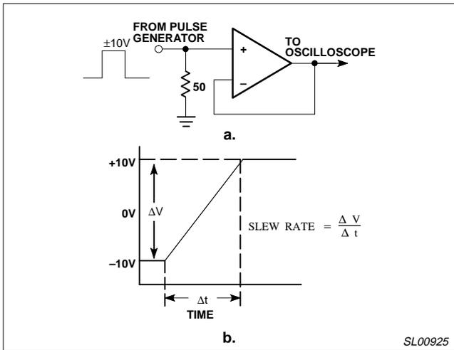
Figure 12. Measuring Slew
