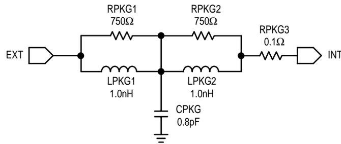
Figure 4. Package Model Schematic
