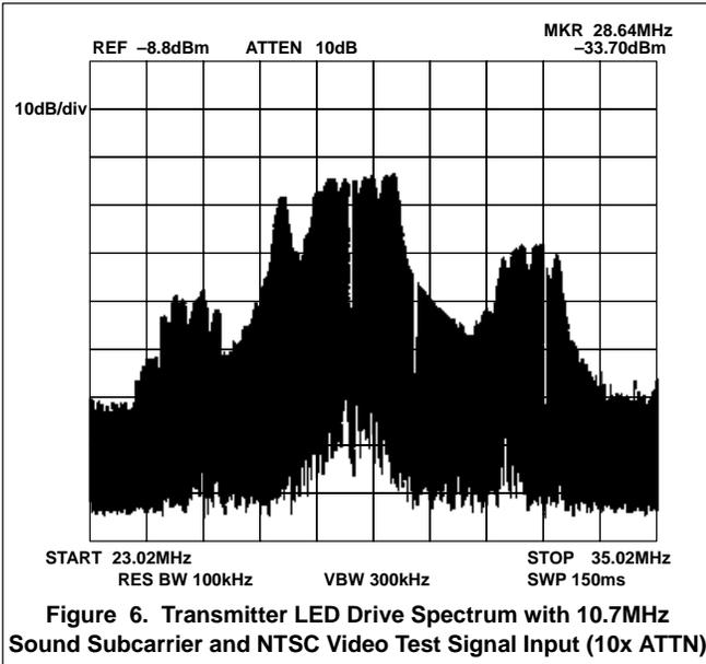
Figure 6. Transmitter LED Drive Spectrum with 10.7MHz Sound Subcarrier and NTSC Video Test Signal Input (10x ATTN)
