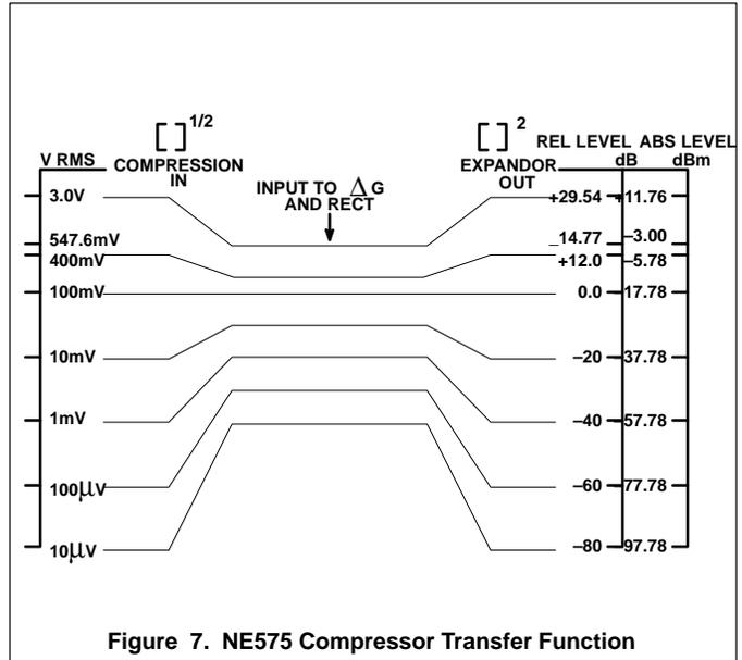
Figure 7. NE575 Compressor Transfer Function
