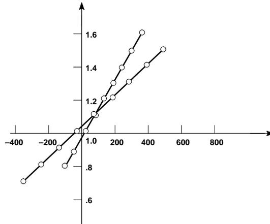
Figure 3. NE564 VCO Transfer Function,  $K_O$
