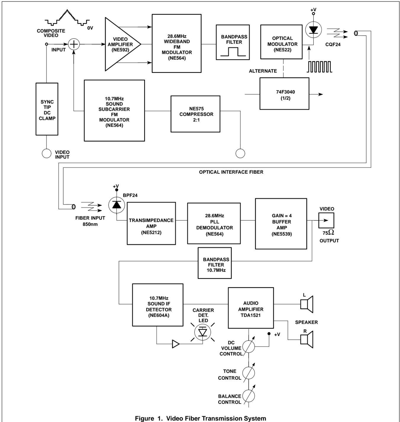
Figure 1. Video Fiber Transmission System
