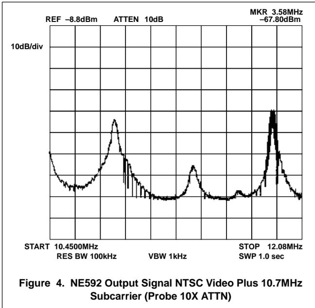
Figure 4. NE592 Output Signal NTSC Video Plus 10.7MHz Subcarrier (Probe 10X ATTN)
