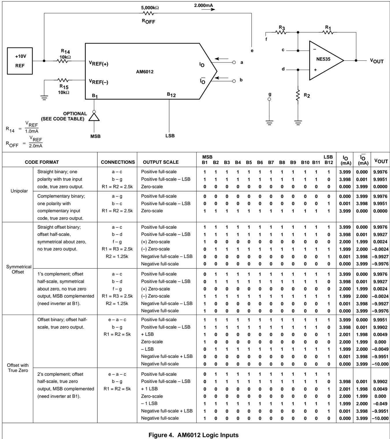
Figure 4. AM6012 Logic Inputs
