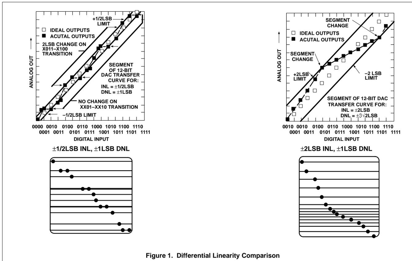
Figure 1. Differential Linearity Comparison
