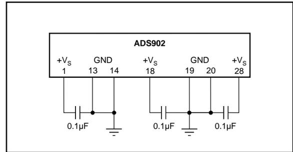
FIGURE 9. Recommended Bypassing for Analog Supply Pins.
