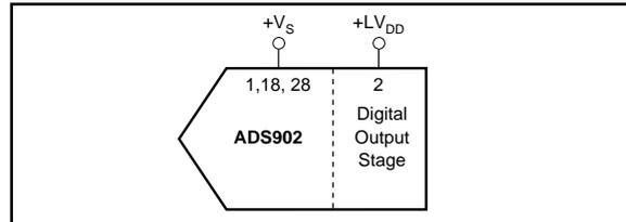
FIGURE 8. Independent Supply Connection for Output Stage.
