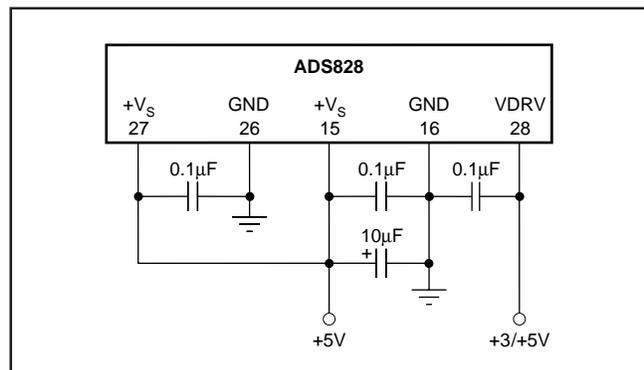
FIGURE 9. Recommended Bypassing for the Supply Pins.
