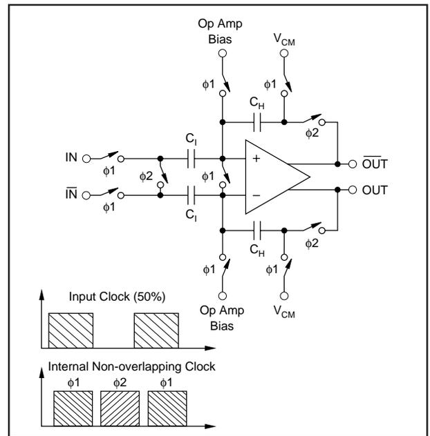
FIGURE 1. Input Track/Hold Configuration with Timing Signals.
