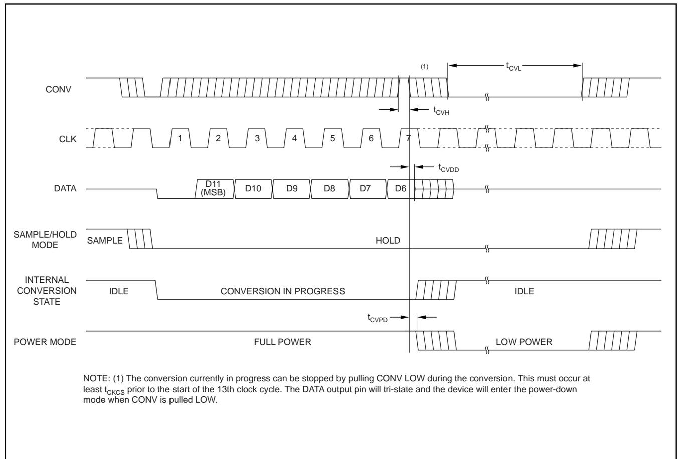
FIGURE 6. Short-cycle Timing.
