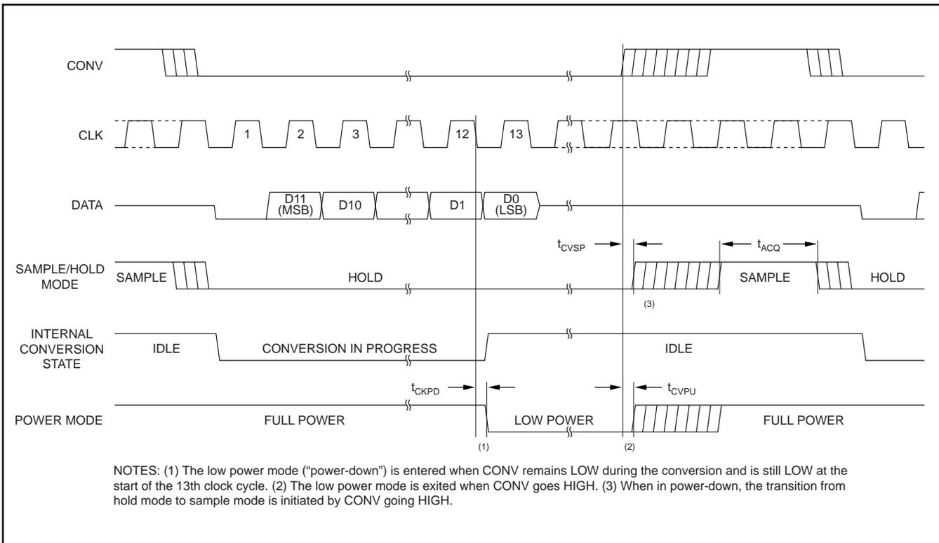
FIGURE 4. Power-down Timing.
