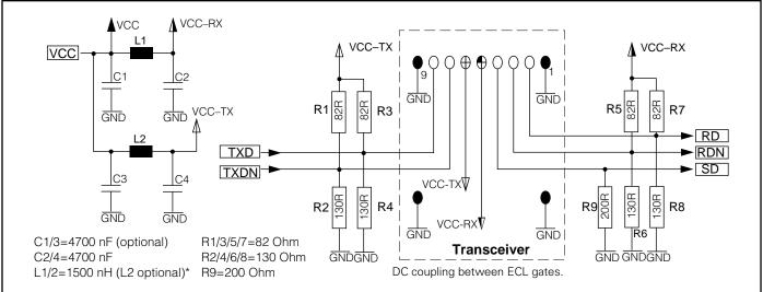
\* Recommended choke is Siemens Matsushita B78108-S1153-K or B78148-S1153-K (Qmin=60, max. DC resistance=0.6 Ohm).
