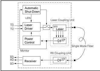
The receiver component converts the optical serial data into PECL compatible electrical data (RD and RDnot). The Signal Detect (SD, active high) shows whether an optical signal is present.
