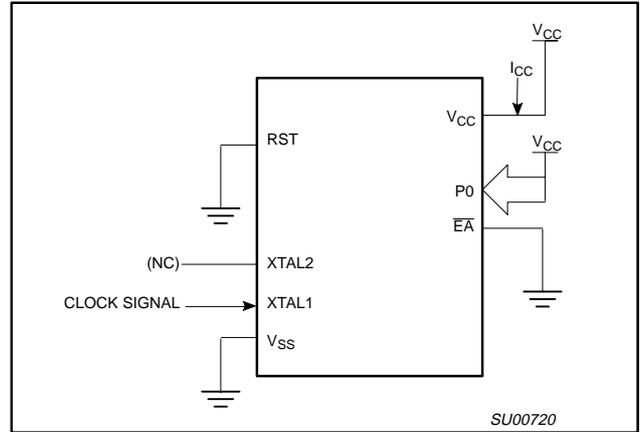
Figure 27.  $I_{CC}$  Test Condition, Idle Mode
