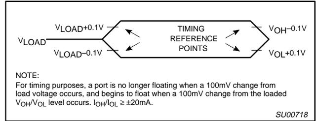
Figure 24. Float Waveform
