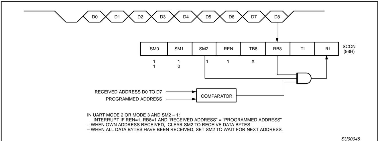
Figure 9. UART Multiprocessor Communication, Automatic Address Recognition
