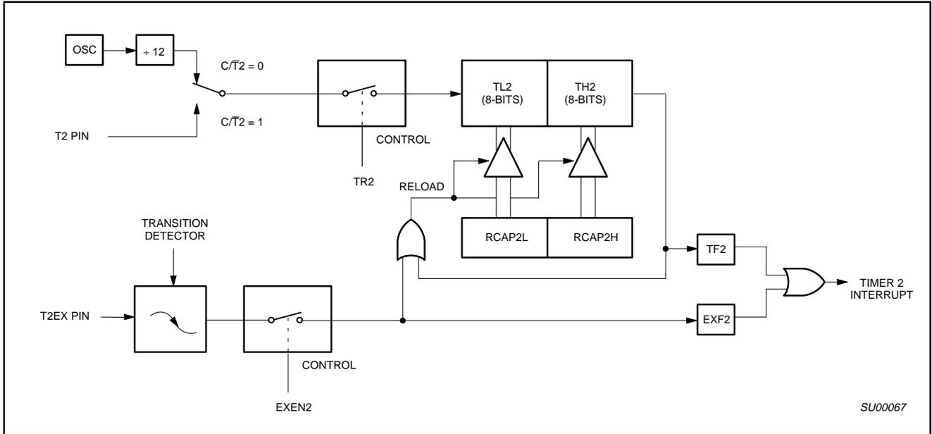
Figure 4. Timer 2 in Auto-Reload Mode (DCEN = 0)
