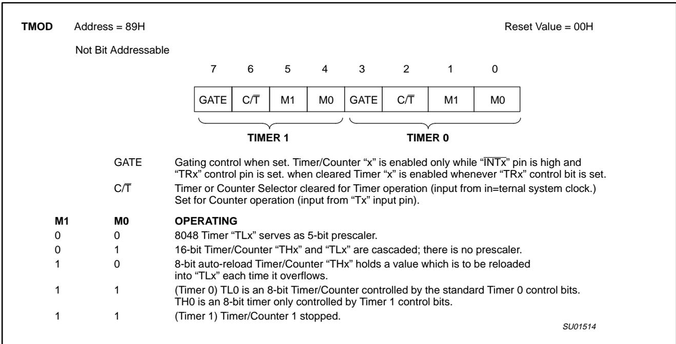
Figure 1. Timer/Counter 0/1 Mode Control (TMOD) Register
