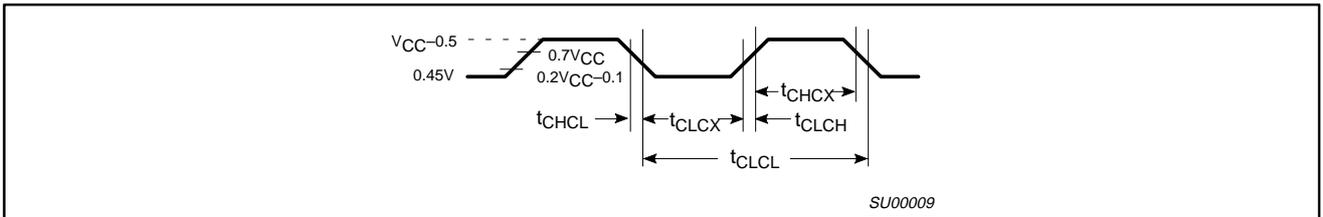
Figure 28. Clock Signal Waveform for  $I_{CC}$  Tests in Active and Idle Modes
