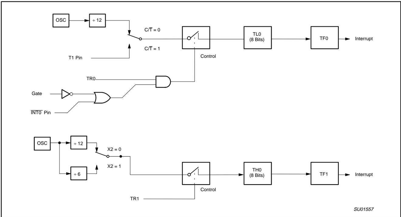
Figure 5. Timer/Counter 0 Mode 3: Two 8-Bit Counters
