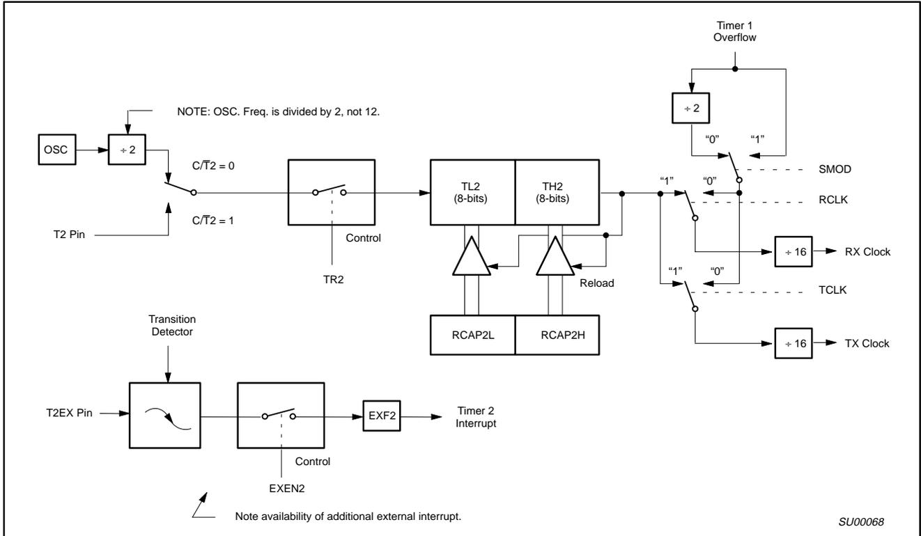
Figure 6. Timer 2 in Baud Rate Generator Mode
