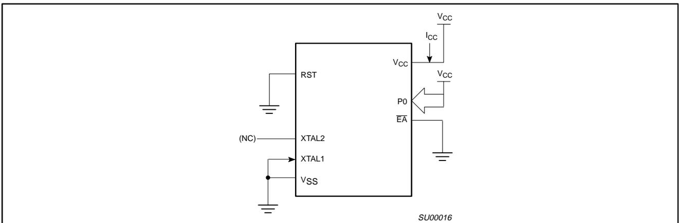
Figure 29.  $I_{CC}$  Test Condition, Power Down Mode
