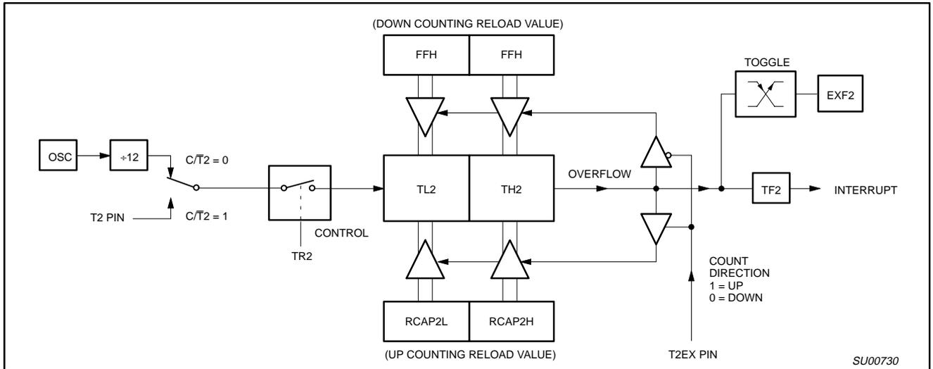
Figure 5. Timer 2 Auto Reload Mode (DCEN = 1)
