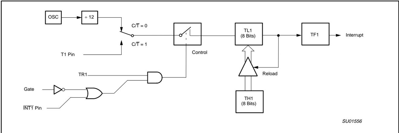
Figure 4. Timer/Counter 0/1 Mode 2: 8-Bit Auto-Load (Timer 1 shown)
