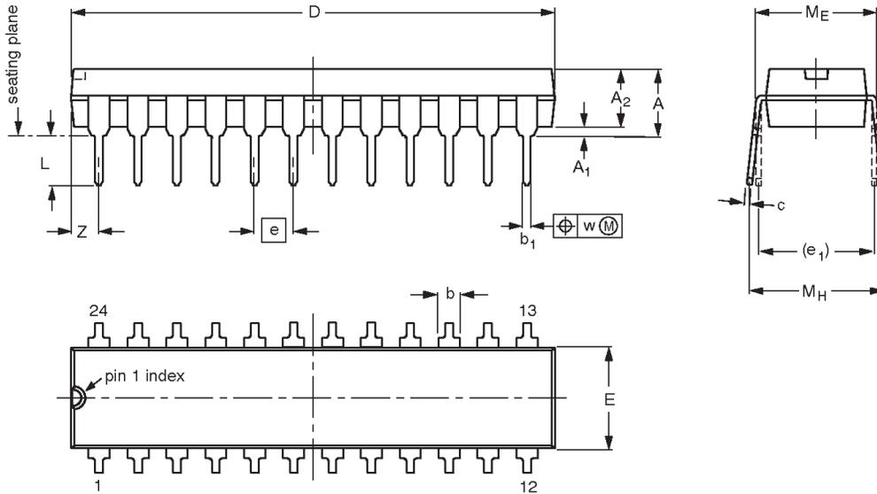
**DIMENSIONS (millimetre dimensions are derived from the original inch dimensions)**
