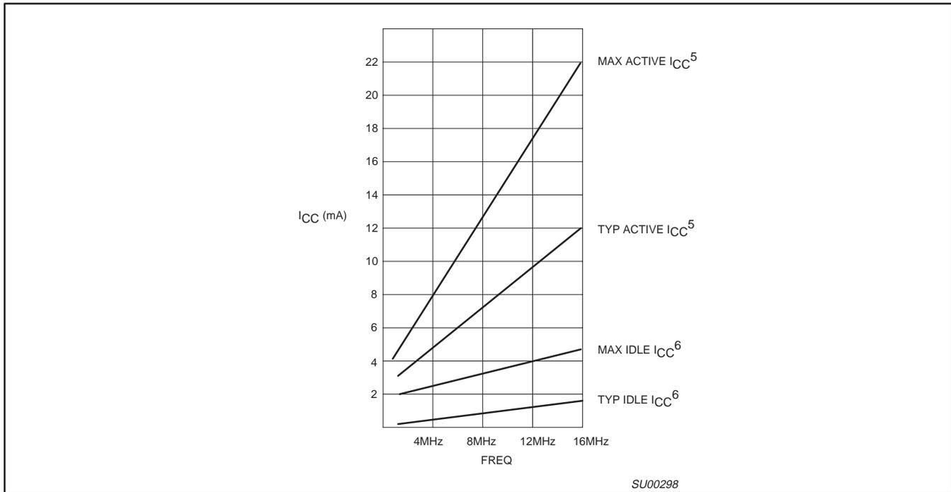
**Figure 2. I<sub>CC</sub> vs. FREQ**
