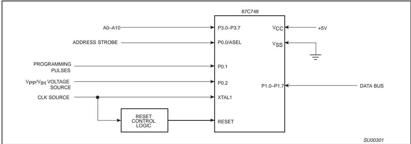
Figure 5. Programming Configuration
