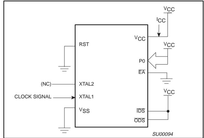
Figure 15.  $I_{CC}$  Test Condition, Idle Mode
