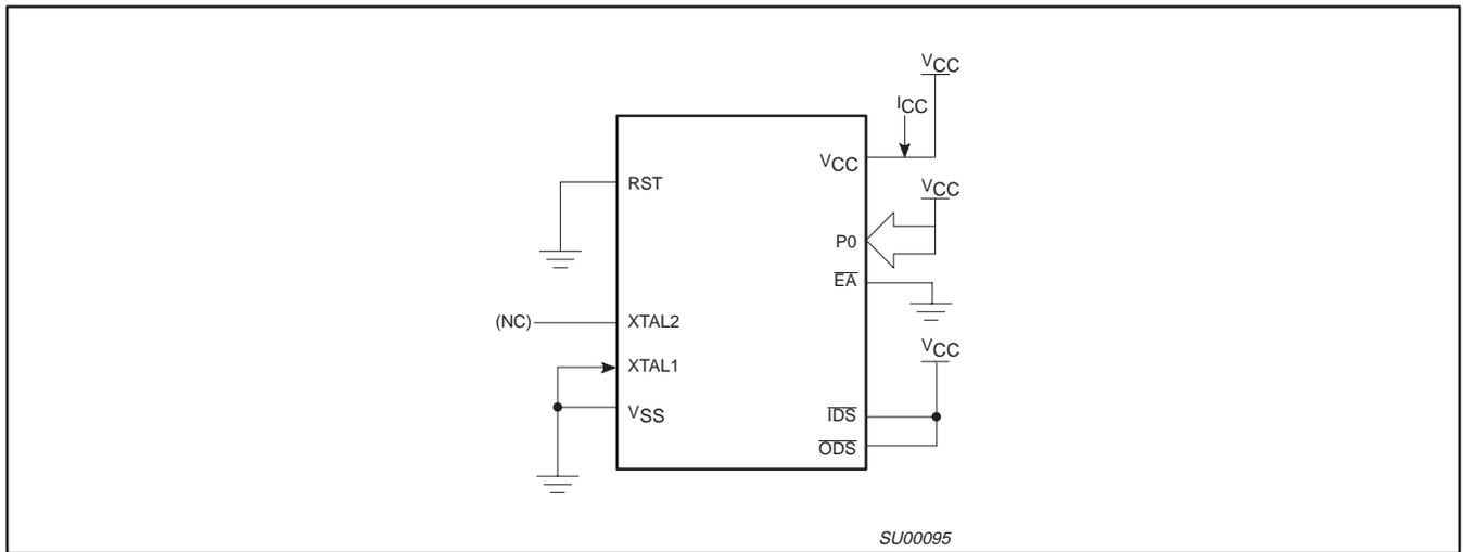
Figure 17.  $I_{CC}$  Test Condition, Power Down Mode
