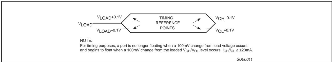
Figure 12. Float Waveform
