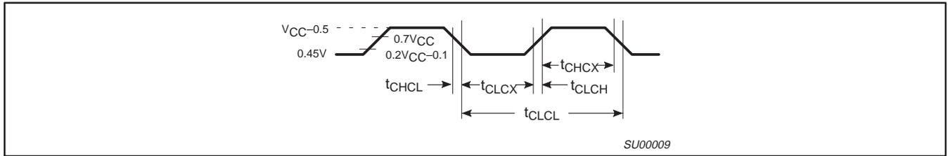
Figure 16. Clock Signal Waveform for  $I_{CC}$  Tests in Active and Idle Modes
