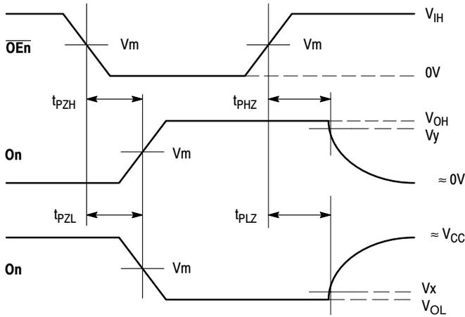
**WAVEFORM 5 - OUTPUT ENABLE AND DISABLE TIMES**
