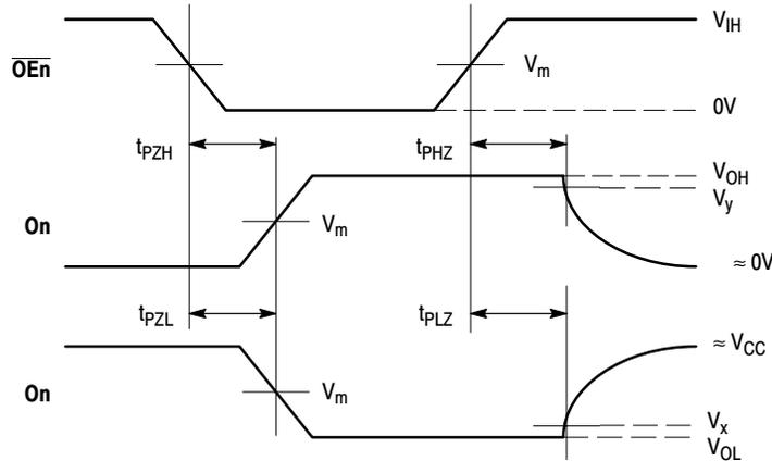
**WAVEFORM 4 - OUTPUT ENABLE AND DISABLE TIMES**
