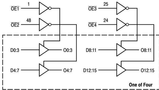
**Figure 2. Logic Diagram**
