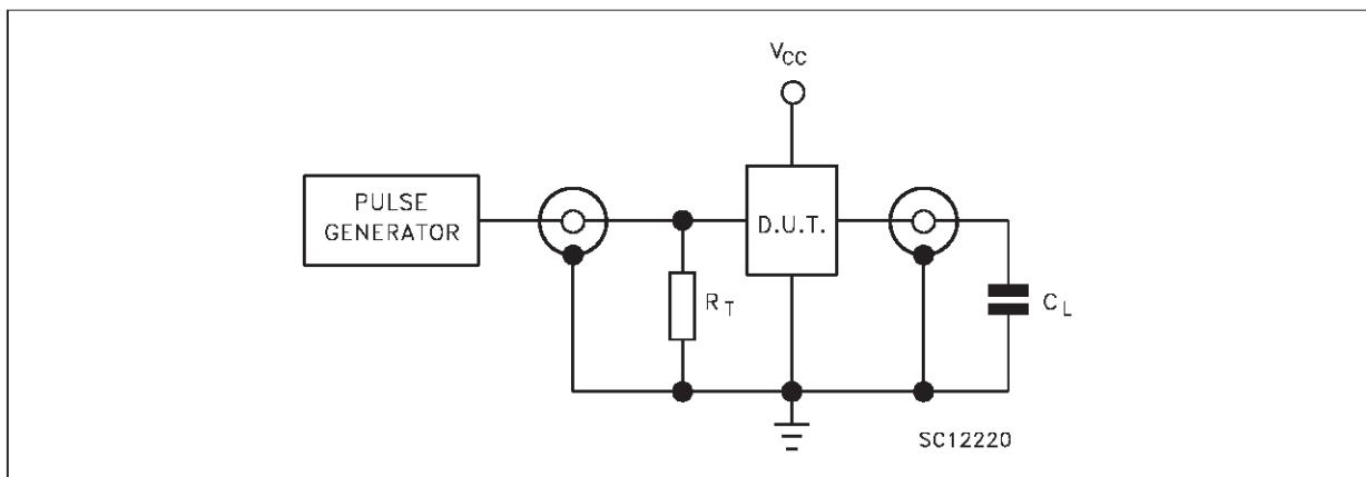
$C_L = 15/50 \text{ pF}$  or equivalent (includes jig and probe capacitance) $R_T = Z_{out}$  of pulse generator (typically  $50\Omega$ )
