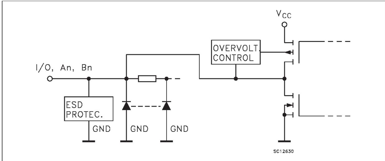
INPUT EQUIVALENT CIRCUIT
