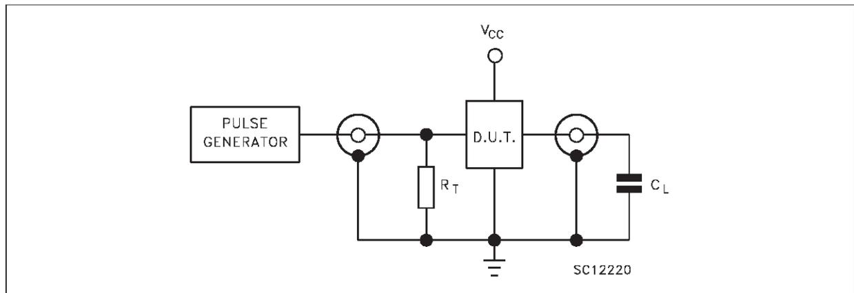
C<sub>L</sub> = 15/50 pF or equivalent (includes jig and probe capacitance)
