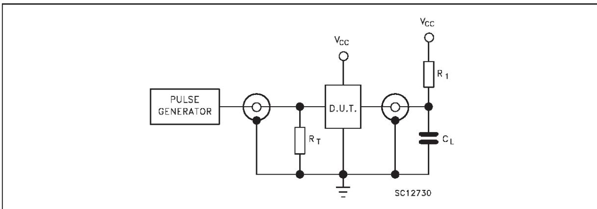
C<sub>L</sub> = 15/50 pF or equivalent (includes jig and probe capacitance)R<sub>L</sub> = R<sub>1</sub> = 1KΩ or equivalentR<sub>T</sub> = Z<sub>out</sub> of pulse generator (typically 50Ω)
