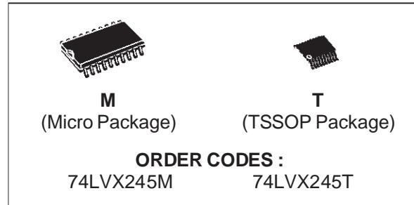
of data transmission is determined by DIR input. The enable input  $\bar{G}$  can be used to disable the device so that the buses are effectively isolated. All inputs and outputs are equipped with protection circuits against static discharge, giving them 2KV ESD immunity and transient excess voltage.
