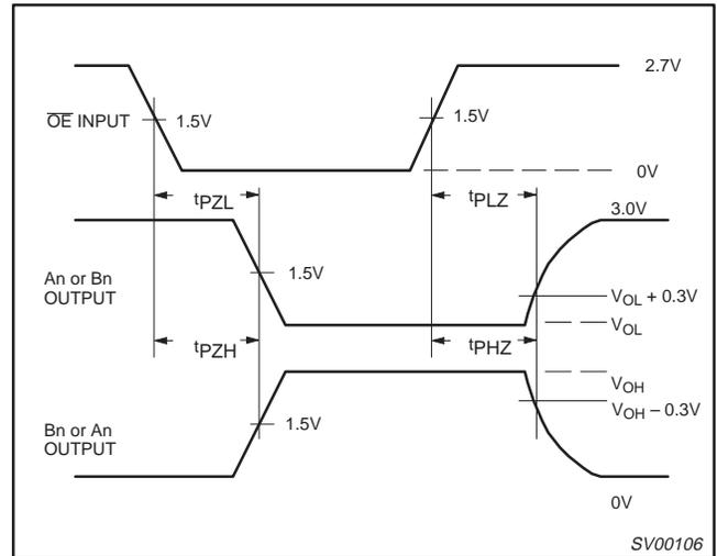
Waveform 2. 3-State Output Enable and Disable Times
