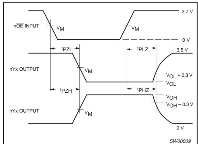
Waveform 2. 3-State Output Enable and Disable Times
