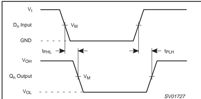
Figure 1. Input ( $D_n$ ) to output ( $Q_n$ ) propagation delays.
