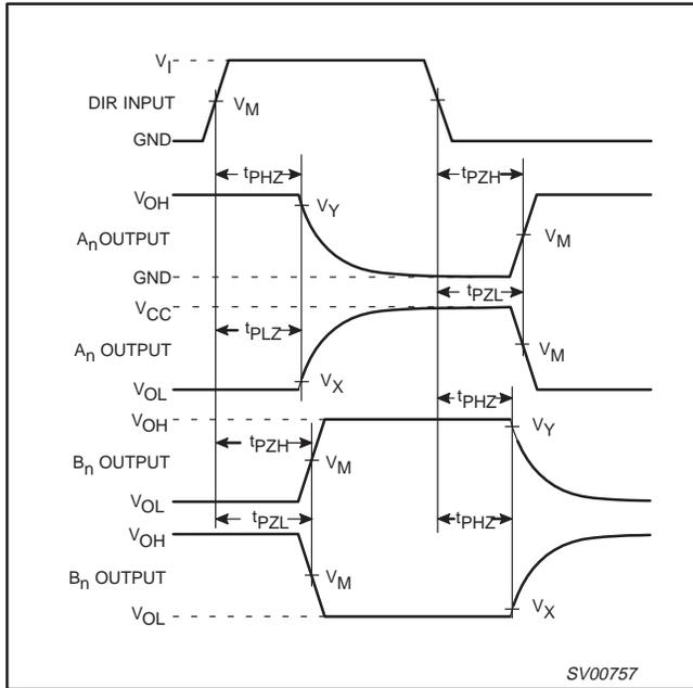
Figure 5. Input DIR to output A<sub>n</sub>, B<sub>n</sub> 3-State enable and disable times.
