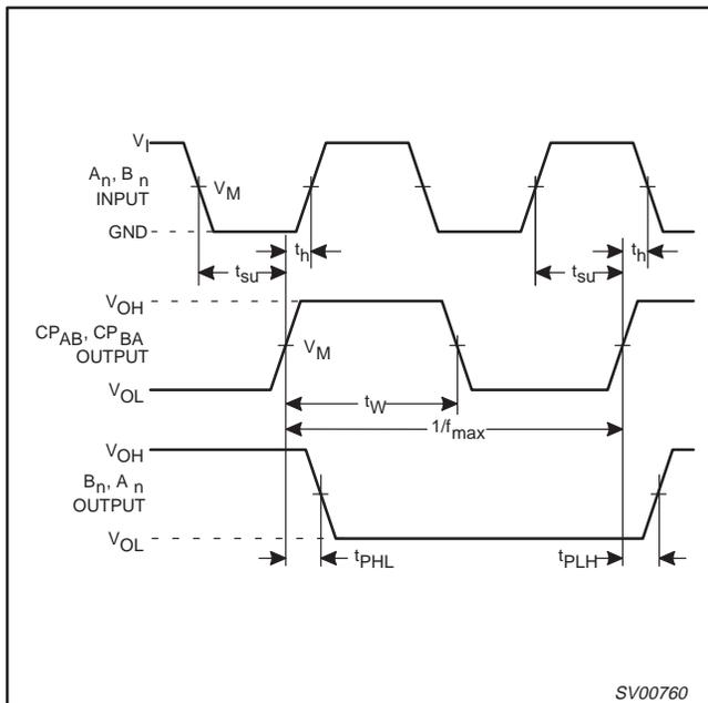
Figure 2.  $A_n, B_n$  to  $CP_{AB}, CP_{BA}$  set-up and hold times, clock  $CP_{AB}, CP_{BA}$  pulse width, maximum clock pulse frequency and the  $CP_{AB}, CP_{BA}$  to output  $B_n, A_n$  propagation delays.
