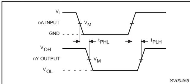
Figure 1. Input (nA) to output (nY) propagation delays.
