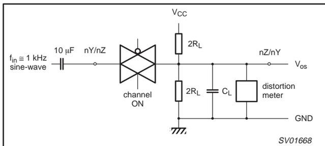
**Figure 10. Test circuit for measuring sine-wave distortion.**
