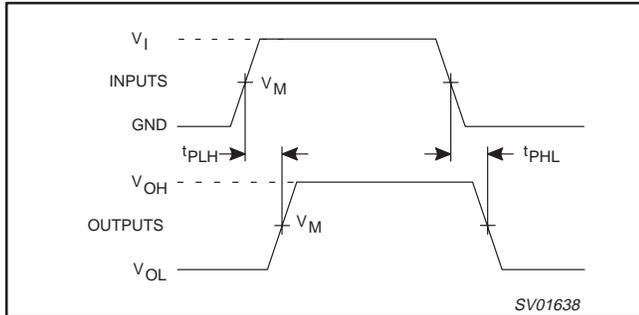
Figure 12. Input ( $V_{1s}$ ) to output ( $V_{0s}$ ) propagation delays.
