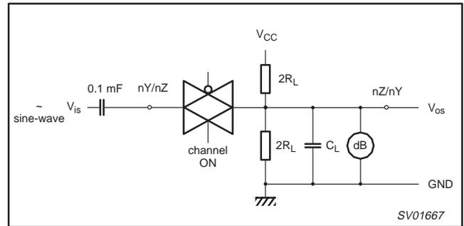
**Figure 9. Test circuit for measuring minimum frequency response.**
