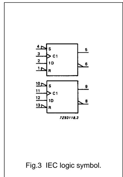
Dual D-type flip-flop with set and reset;
