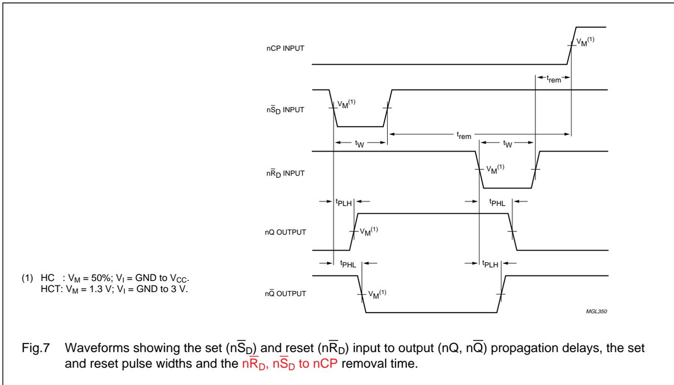
Dual D-type flip-flop with set and reset;
