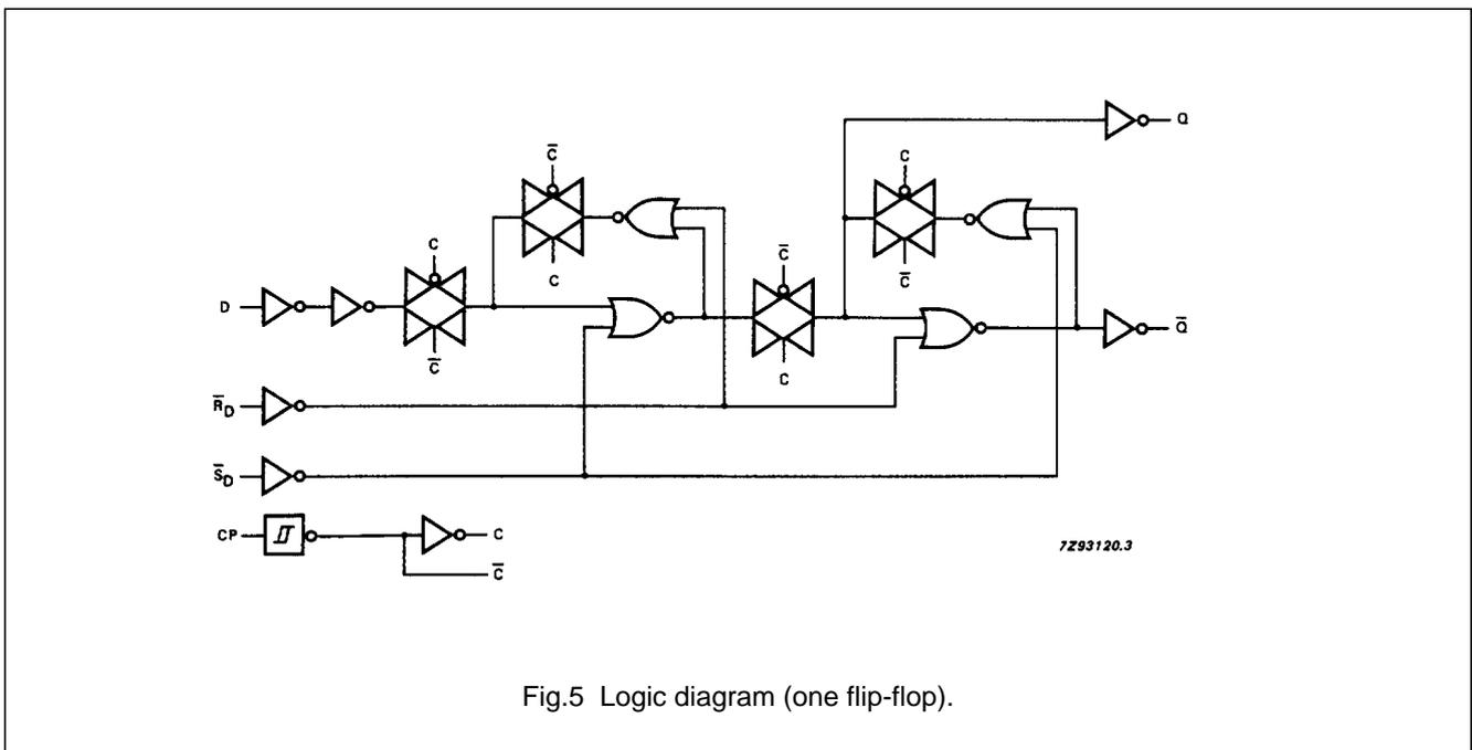
Fig.5 Logic diagram (one flip-flop).
