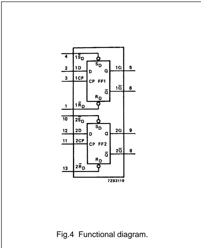
Fig.4 Functional diagram.
