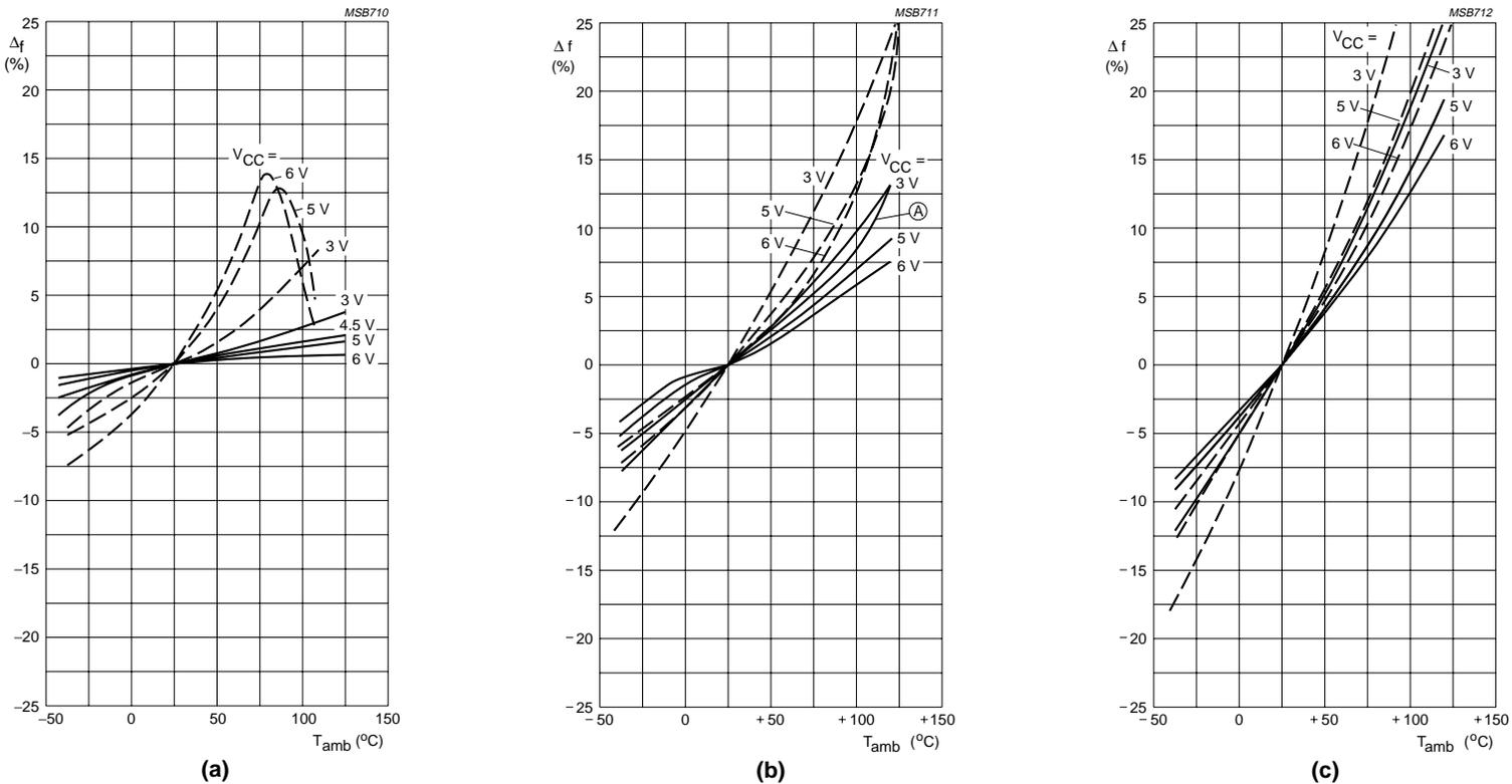
Fig.16 Frequency stability of the VCO as a function of ambient temperature with supply voltage as a parameter.
