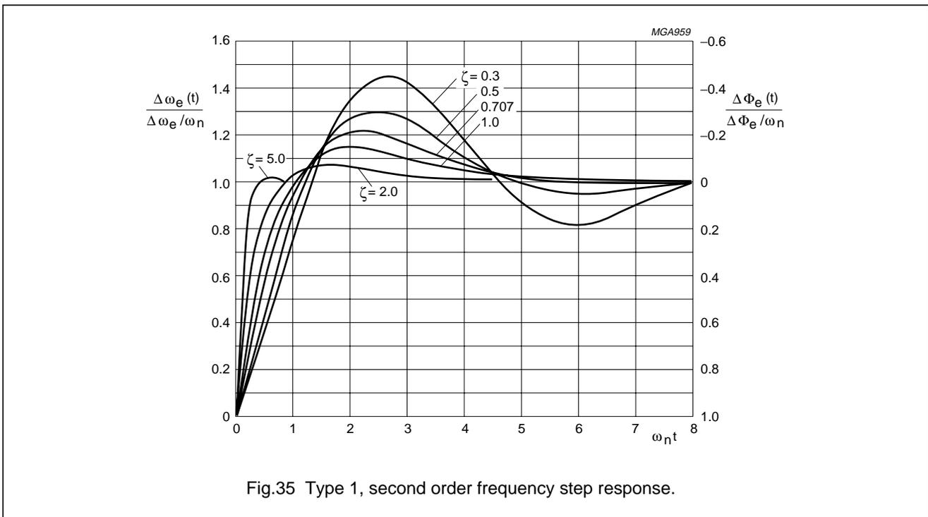
Since the output frequency is proportional to the VCO control voltage, the PLL frequency response can be observed with an oscilloscope by monitoring pin 9 of the VCO. The average frequency response, as calculated by the Laplace method, is found experimentally by smoothing this voltage at pin 9 with a simple RC filter, whose time constant is long compared to the phase detector sampling rate but short compared to the PLL response time.
