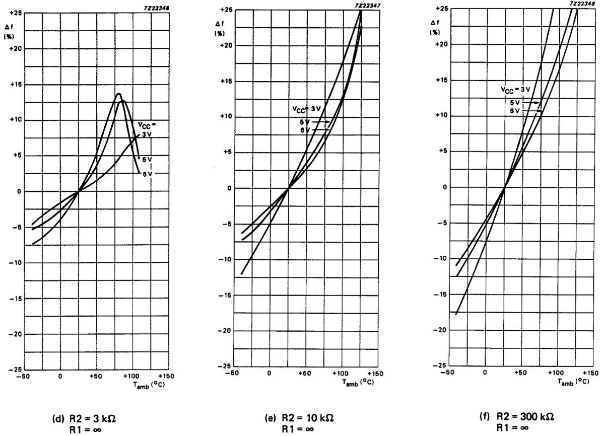
To obtain optimum temperature stability,  $C_1$  must be as small as possible, but larger than 100 pF.
