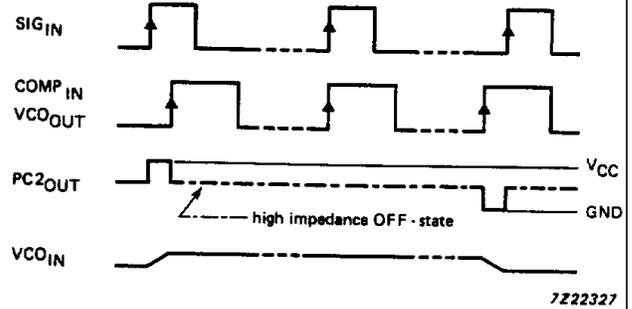
Fig.9 Typical waveforms for PLL using phase comparator 2, loop locked at  $f_0$ .
