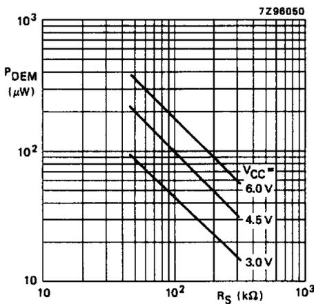
Fig.22 Typical dc power dissipation of demodulator section as a function of  $R_S$ :  $R_1 = R_2 = \infty$ ;
