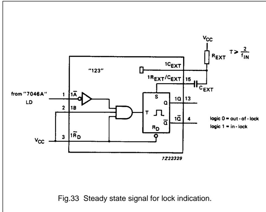
Fig.33 Steady state signal for lock indication.
