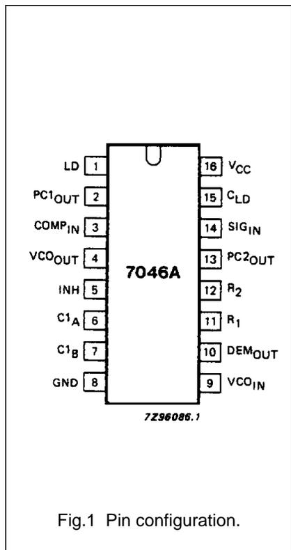
Fig.1 Pin configuration.
