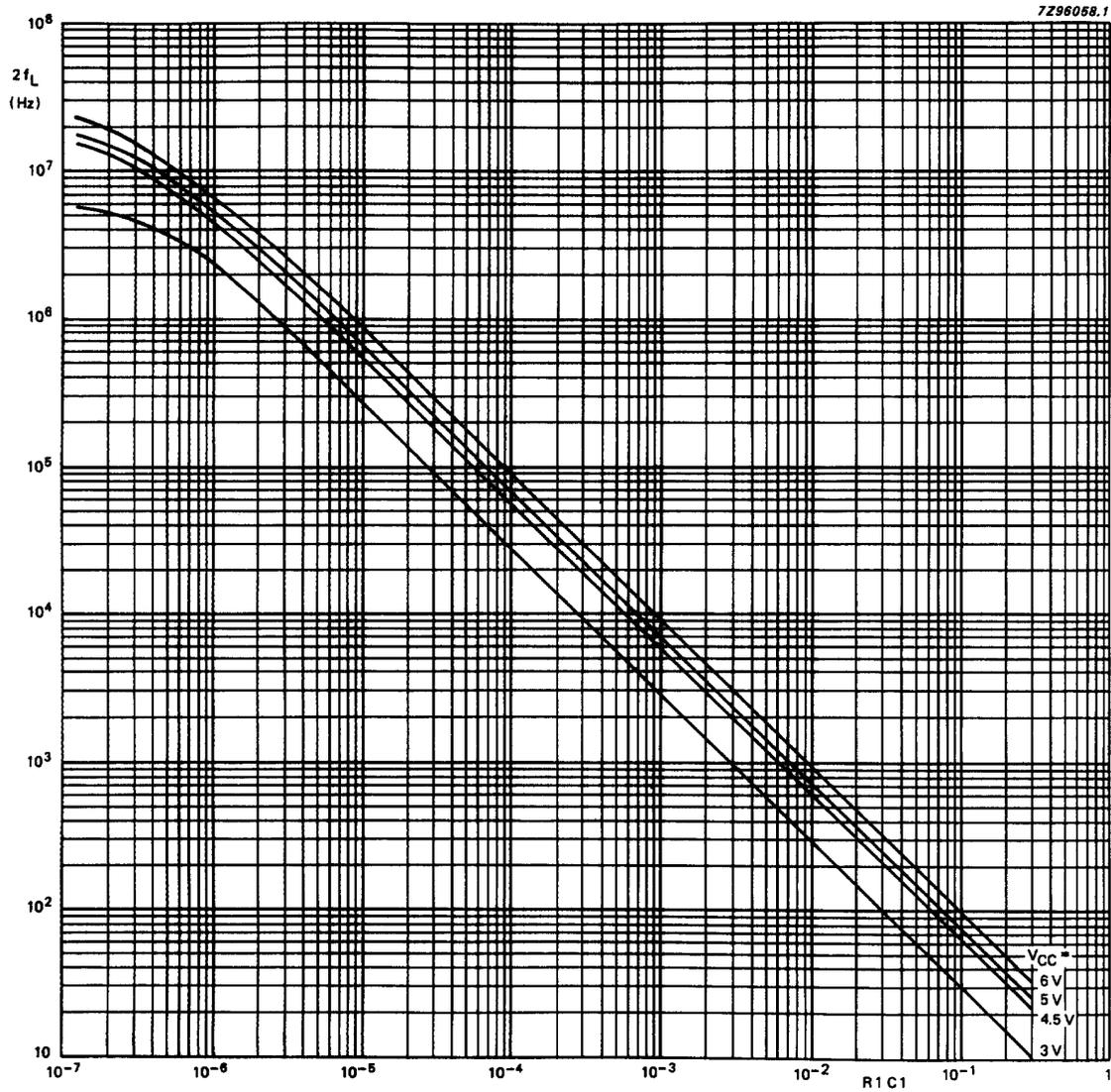
Fig.29 Typical frequency lock range ( $2f_L$ ) versus the product  $R1C1$ :  $V_{VCOIN}$  range = 0.9 to  $(V_{CC} - 0.9)$  V;  $R2 = \infty$ ; VCO gain:
