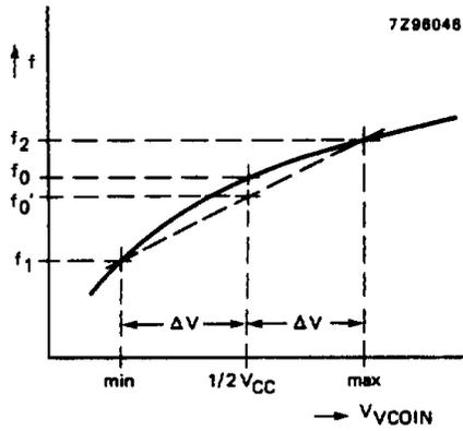
Fig.18 Definition of VCO frequency linearity:
