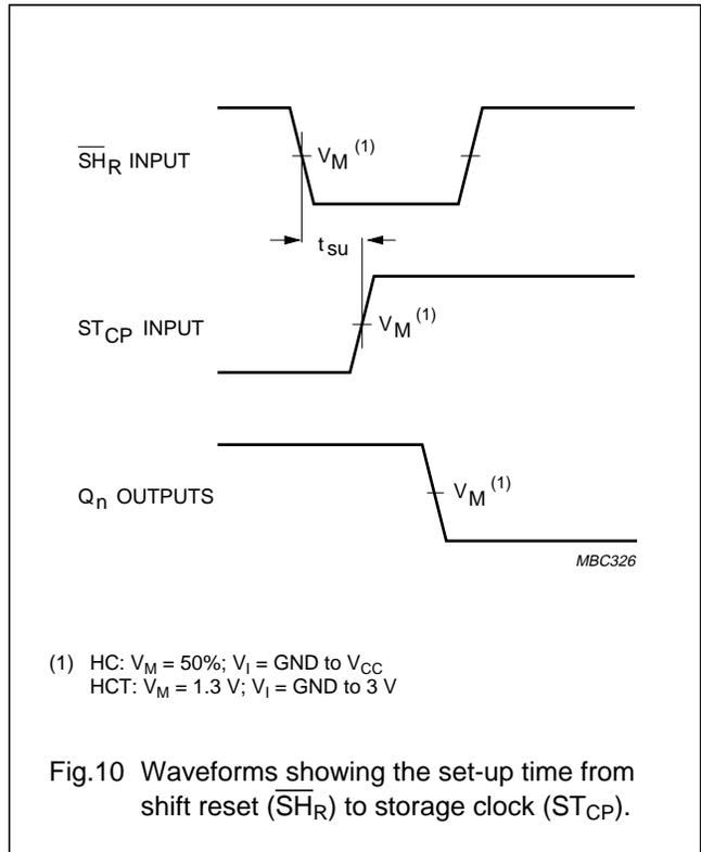
8-bit shift register with output register
