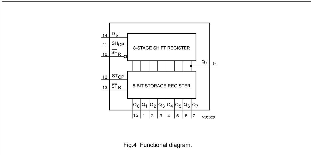
Fig.4 Functional diagram.
