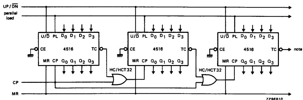
Ripple clocking mode: the UP/DN control can be changed at any count. The only restriction on changing the UP/DN control is that the clock input to the first counting stage must be "HIGH". For cascading counters operating in a fixed up-count or down-count mode, the OR gates are not required between stages and  $\overline{TC}$  is connected directly to the CP input of the next stage with  $\overline{CE}$  grounded.
