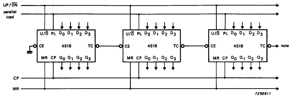
Terminal count ( $\overline{TC}$ ) lines at the 2nd, 3rd, etc. stages may have a negative-going glitch pulse resulting from differential delays of different 4516s. These negative-going glitches do not affect proper 4516 operation. However, if the terminal count signals are used to trigger other edge-sensitive logic devices, such as flip-flops or counters, the terminal count signals should be gated with the clock signal using a 2-input OR gate such as HC/HCT32.
