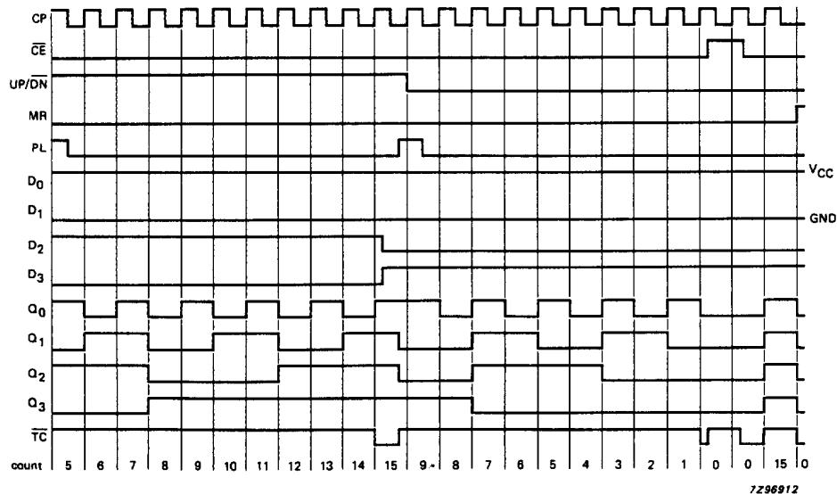
Fig.5 Timing diagram.
