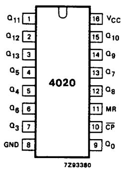
Fig.1 Pin configuration.
