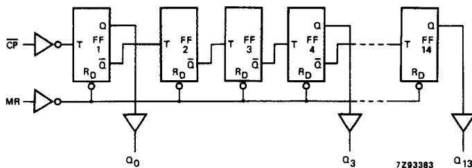
Fig.5 Logic diagram.
