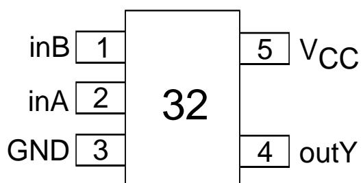
Fig.1 Pin configuration.
