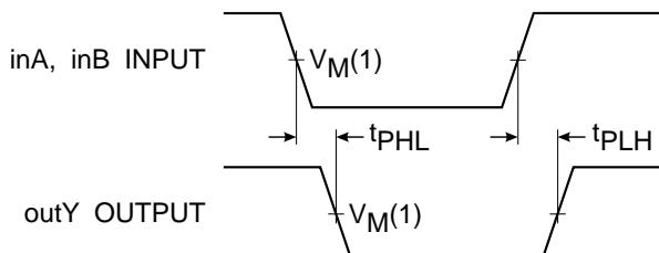
Fig.5 The input (inA, inB) to output (outY) propagation delays.
