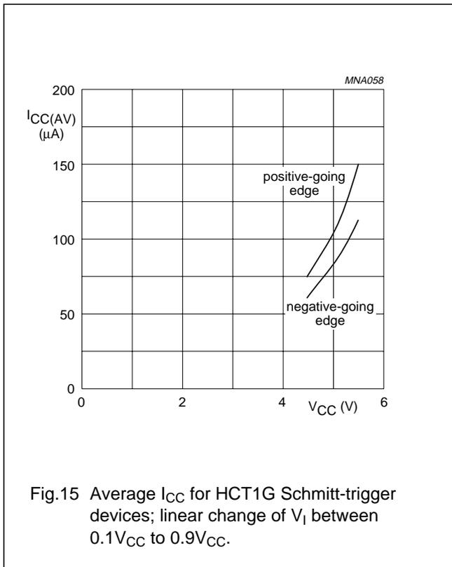
Fig.15 Average  $I_{CC}$  for HCT1G Schmitt-trigger devices; linear change of  $V_I$  between  $0.1V_{CC}$  to  $0.9V_{CC}$ .
