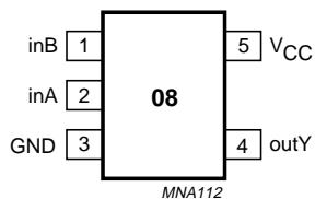
Fig.1 Pin configuration.
