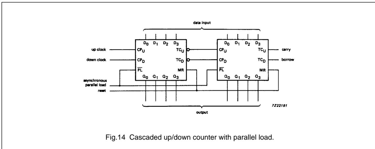
Fig.14 Cascaded up/down counter with parallel load.
