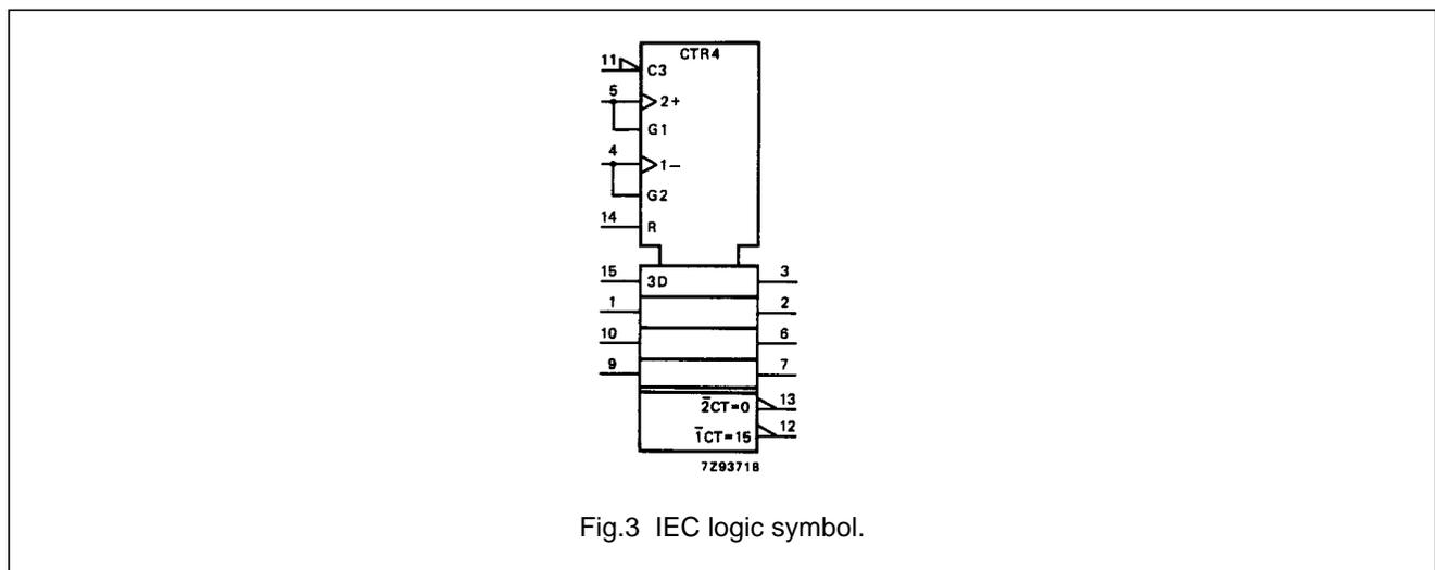
Pre-settable synchronous 4-bit binary
