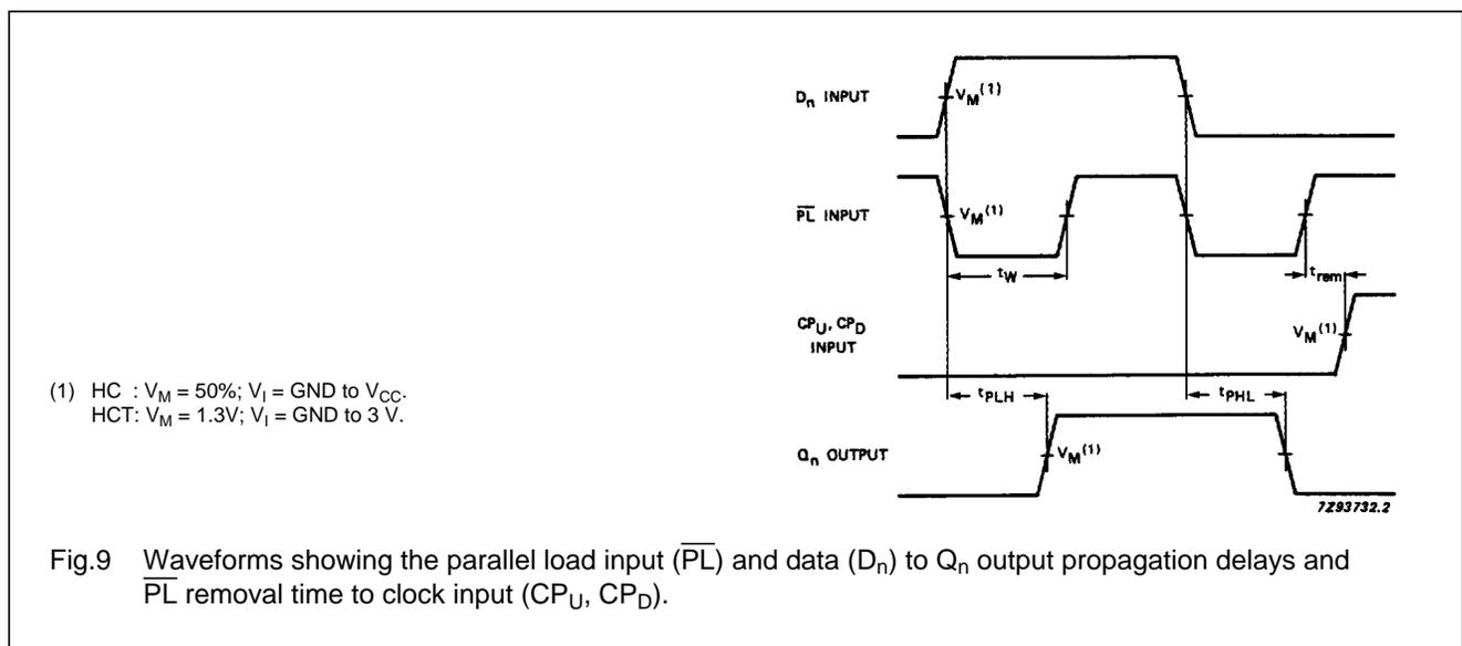
Pre-settable synchronous 4-bit binary up/down counter
