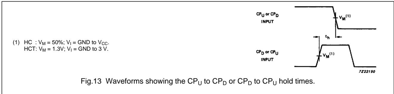
Pre-settable synchronous 4-bit binary up/down counter
