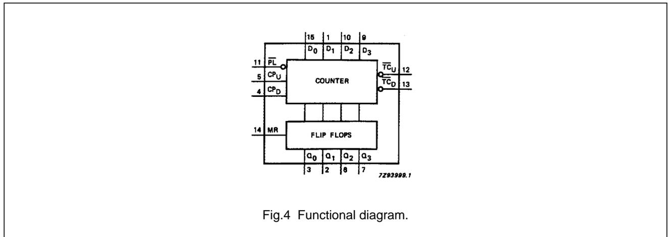
Fig.4 Functional diagram.
