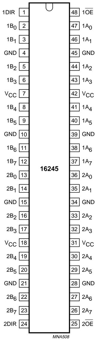
Fig.3 Pin configuration.
