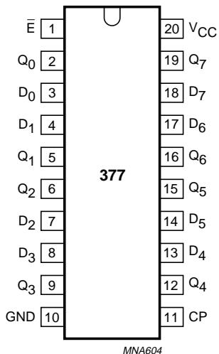
Fig.1 Pin configuration.
