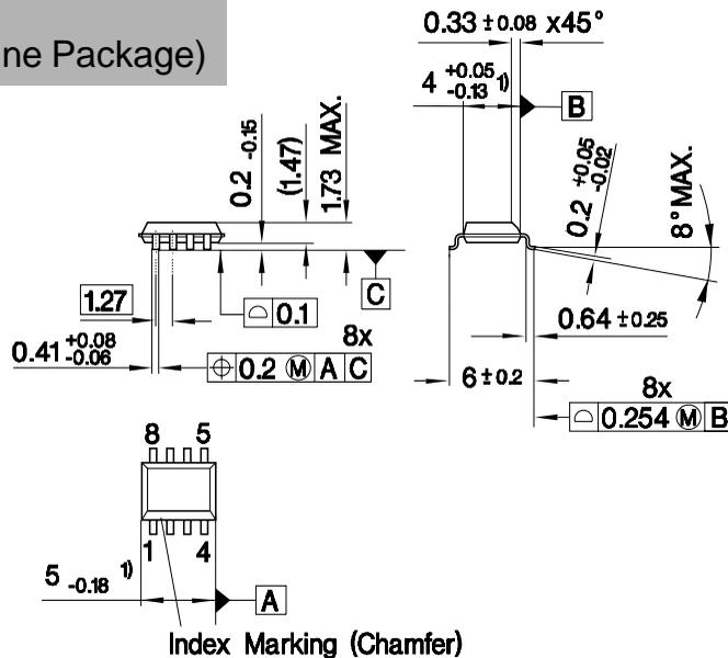
1) Does not include plastic or metal protrusion of 0.15 max. per side
