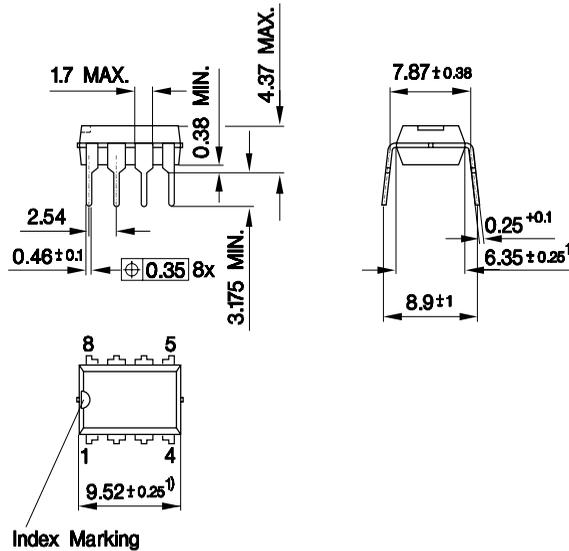
1) Does not include plastic or metal protrusion of 0.25 max. per side
